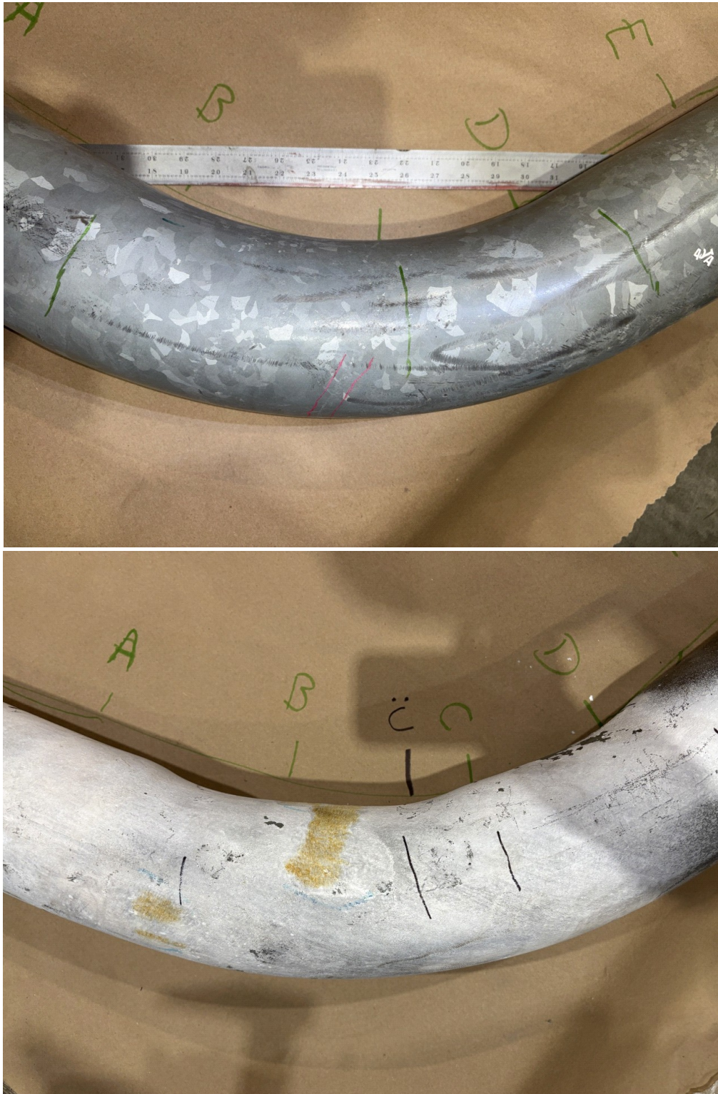
Image 19 – Comparison of the variation of smoothness of the interior bend geometries between two arms from the GEE Gondola.
