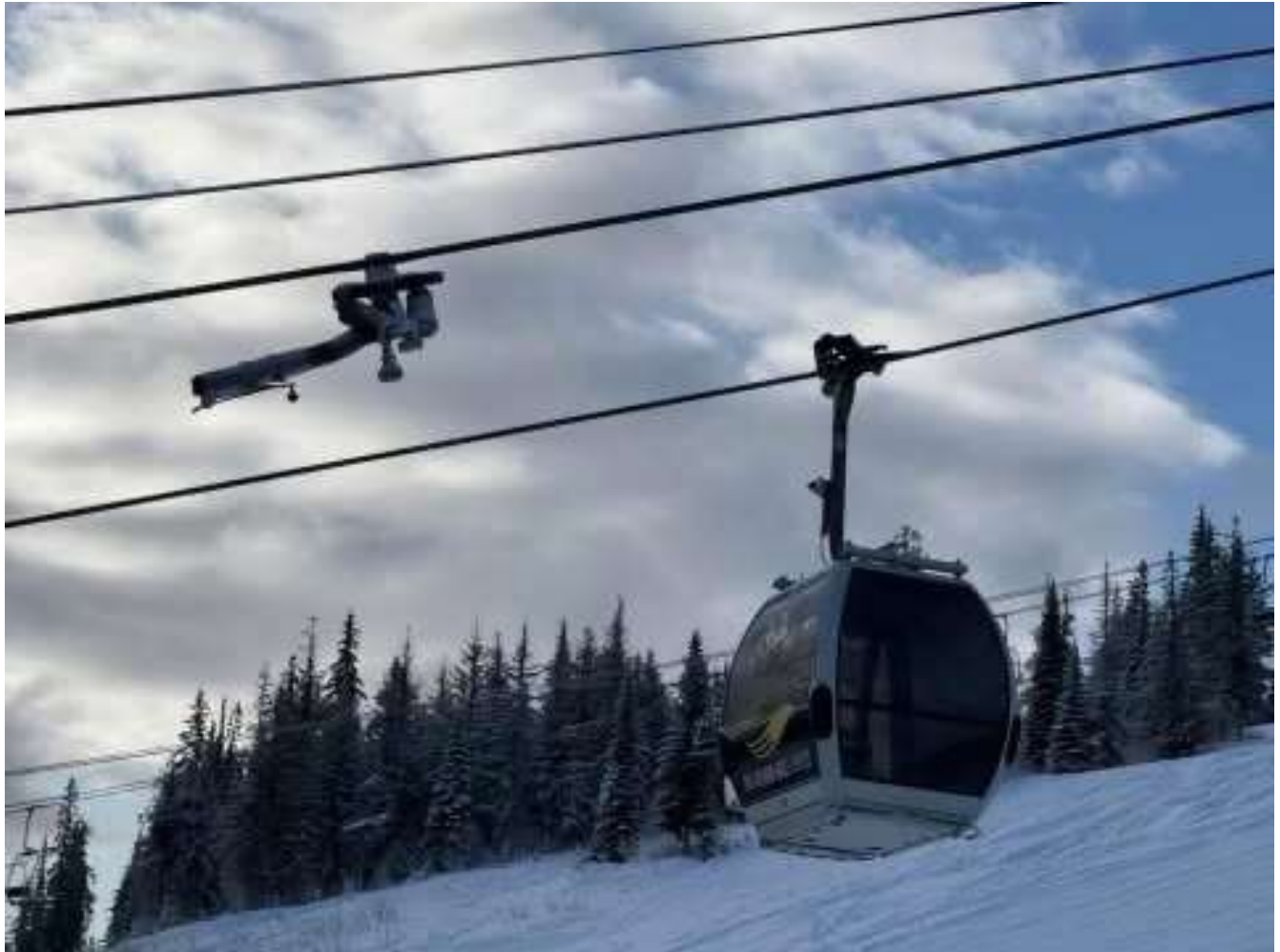
Image 3 - The remaining portion of the hanger arm and grip still connected to the lift line after the incident (Photograph provided by Resorts of the Canadian Rockies)
