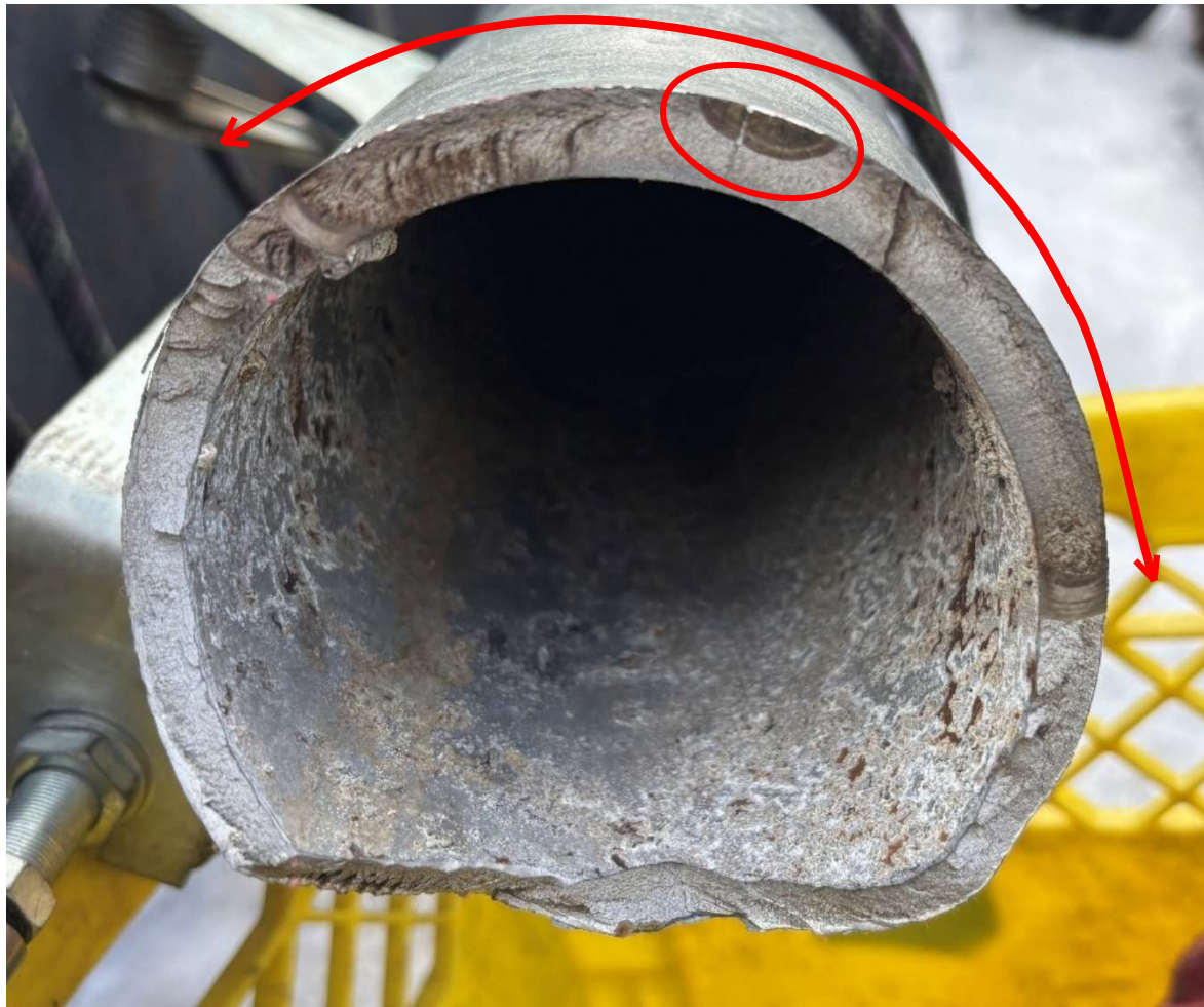
Figure 7 - Overview of the fracture face. Circle – “thumbnail” initiation site. Arrow – Approximate length of the crack present during operation leading up to the incident. Note the colour differences from corrosion products between the “thumbnail”, the first large progression (noted by the arrow), and the bright silver of the fresh fracture face.
