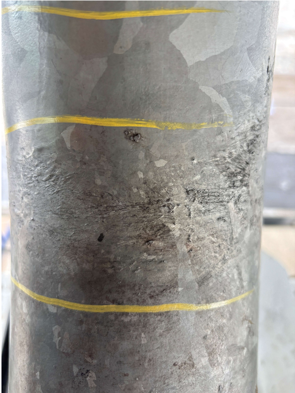
Image 17 – A close up of wrinkling and horizontal lines on another hanger arm during post-incident testing.
