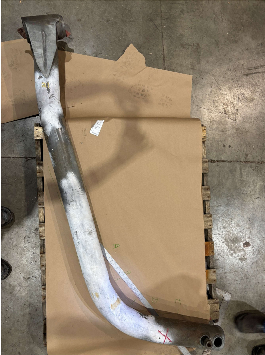
Image 18 – Example of an arm located I the Acuren facility after undergoing extensive MPI testing and documentation.
