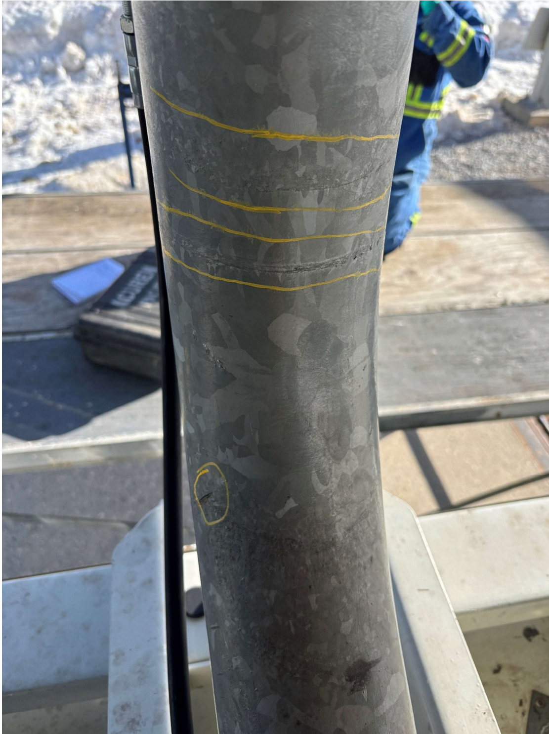
Image 16 – A view of a hanger arm during inspection. Irregularities in the surface including lines, marks, and scrapes are highlighted.
