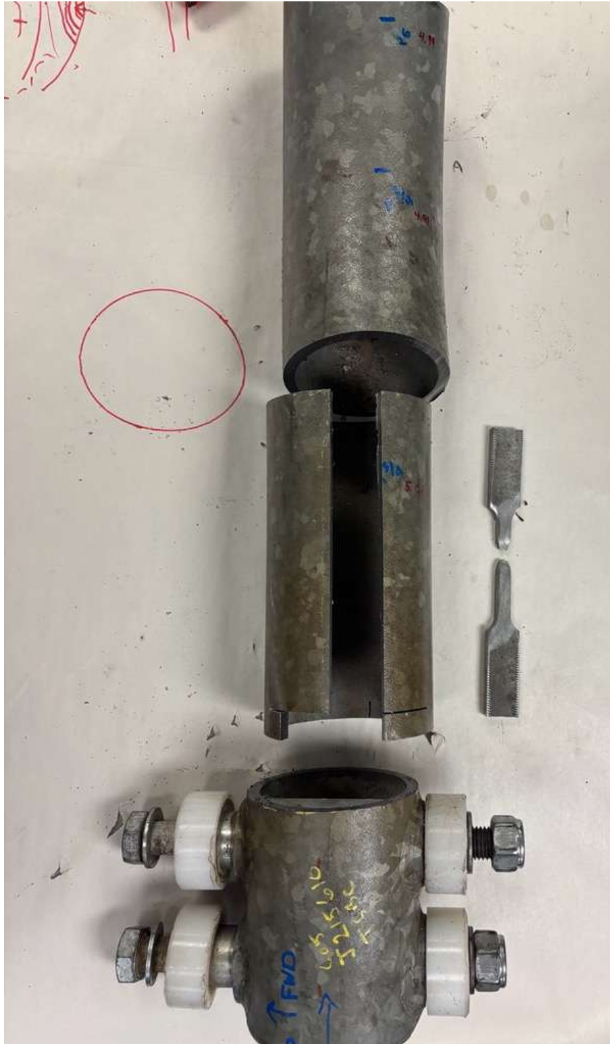
Image 20 – The bottom portion of the failed arm after being sectioned for various tests including metal chemistry, tensile tests, and fracture analysis.
