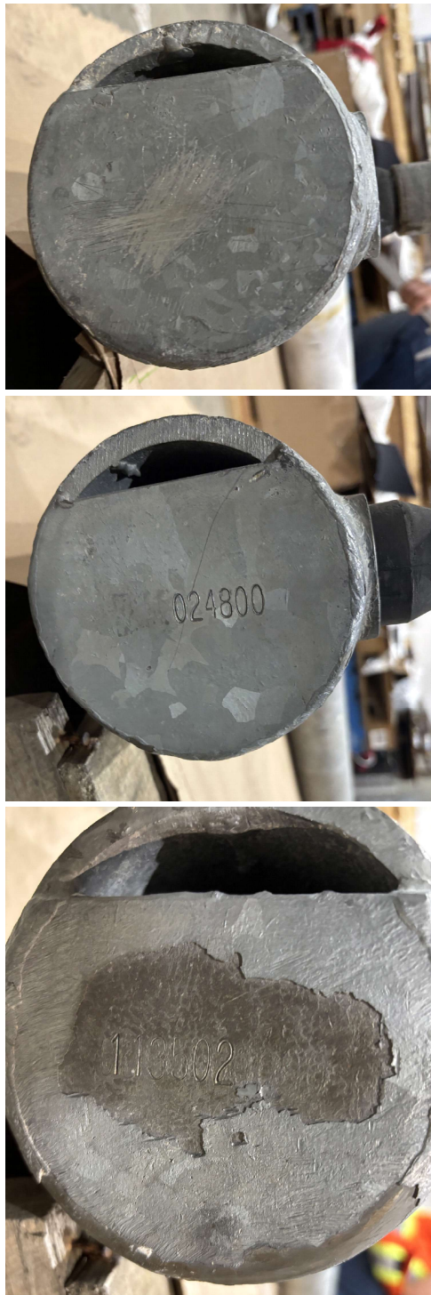
Image 21 – Three arms from the GEE gondola. One with no serial number. One with the serial number stamped on top of the galvanizing. One with the serial number stamped beneath the galvanizing. The arms with numbers were not close to being sequential.
