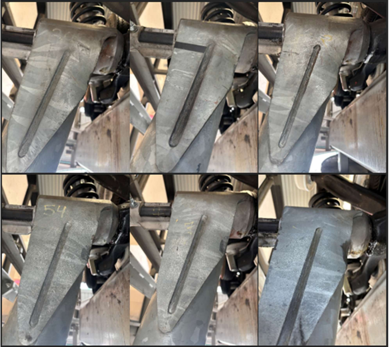
Image 14 – A compilation of severely bent gussets on various GEE gondola hanger arms taken during investigation after the incident.
