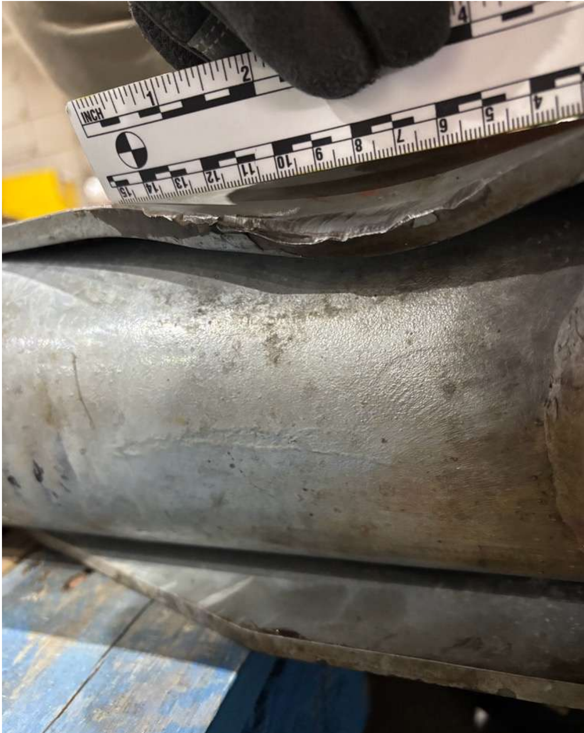
Image 15 - A close up the deformation and damage to the gusset on the failed hanger arm for cabin 15.
