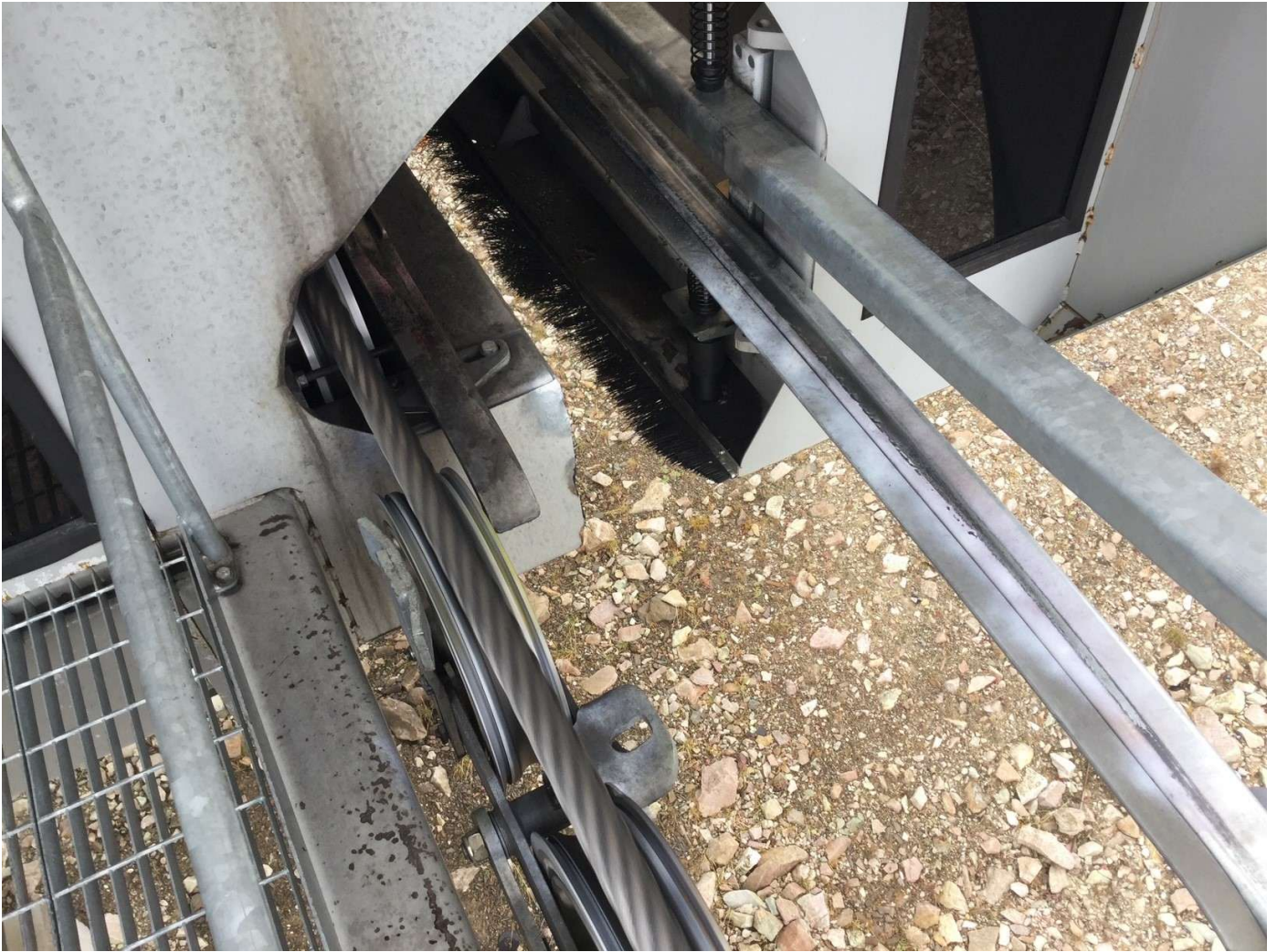
Image 12 – A similar photograph taken by a Safety Officer in 2018, approximately 1 year later. The rubber bumpers are still missing.
