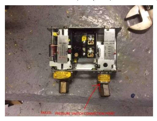
Shows failed pressure switch connection point, Note: the Pressure switch connection fitting has been bent or opened up to show where the crack started.
