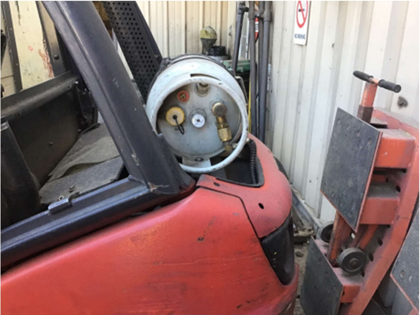
Image 4 – Propane cylinder mounted on the forklift
