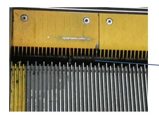
Step piled up on top of another. Visible gap between steps.
