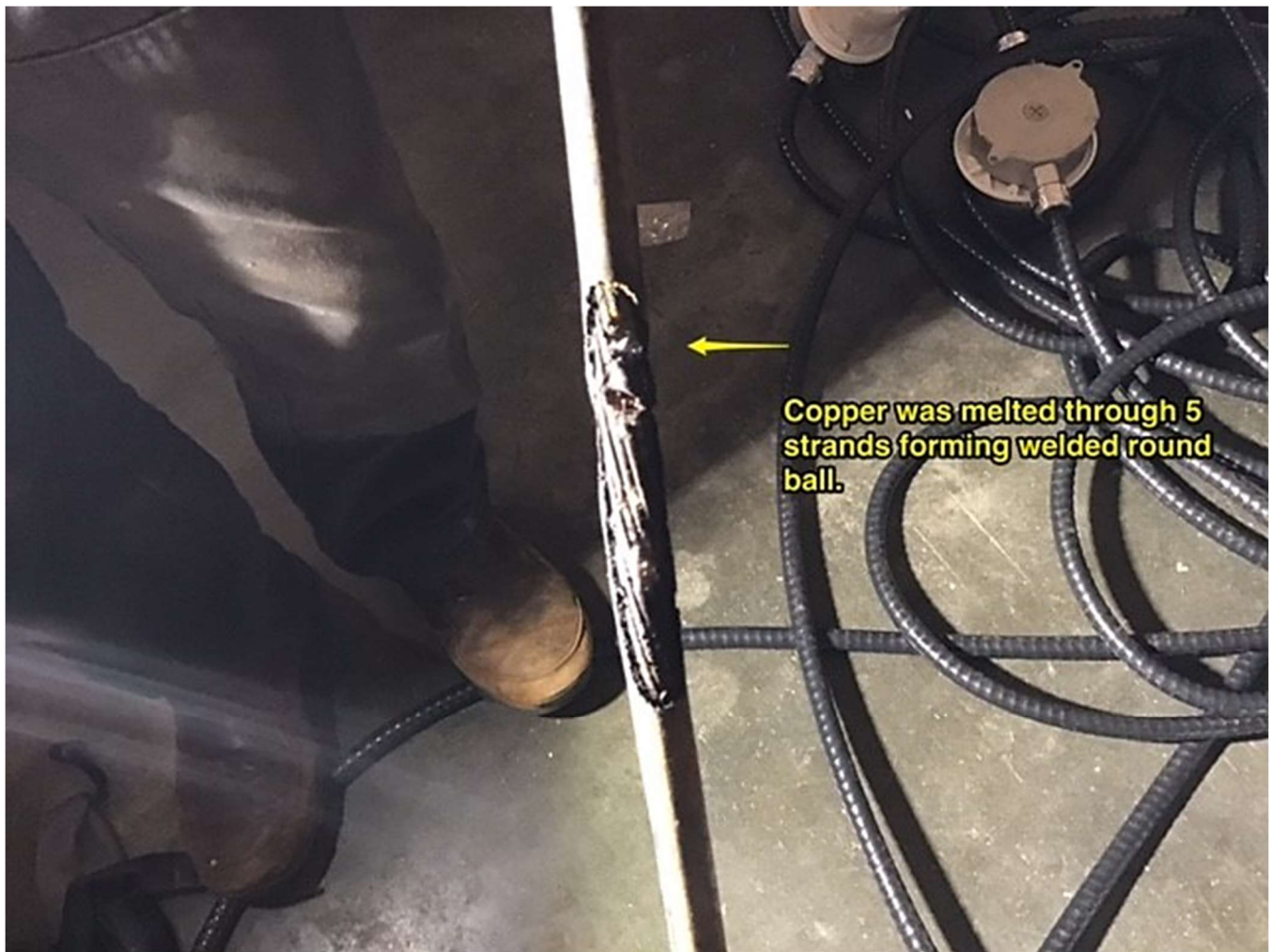
Figure 6 – Close up of melting damage to the uninsulated portion of a line conductor
