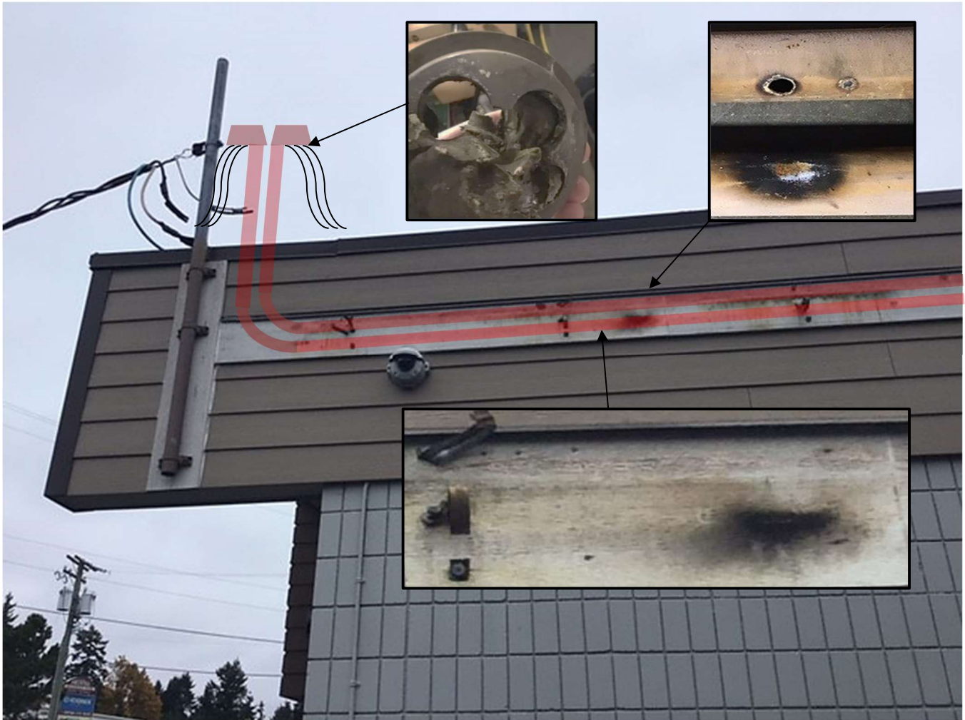
Figure 4 - Location of the parallel metal service conduits (in red). The arcing occurred on the horizontal section of the upper conduit with the smoke mark shown on the backboard (bottom). Damage to the entrance cap openings (top left). Back view of the arcing hole on the damaged conduit and smoke damage on the adjacent conduit (top right).
