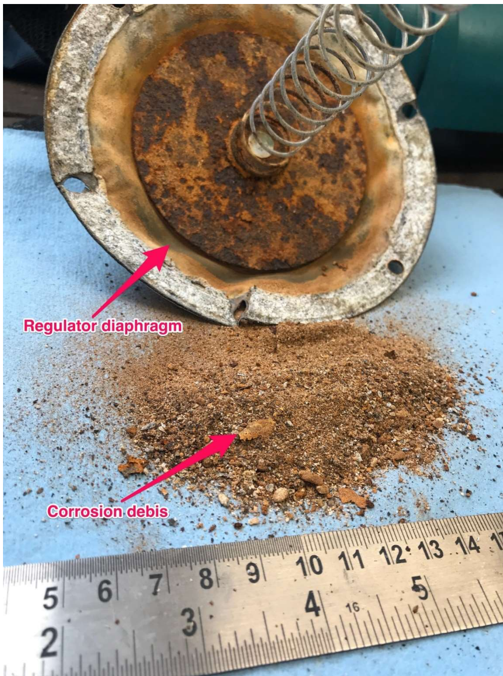
Image #6 Corrosion debris removed from regulator diaphragm
