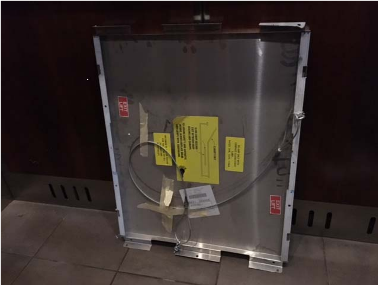
Photo 1- Emergency Escape hatch. Hatch securing cable taped to the interior of the hatch. Photo taken on-site by notifier after incident occurred prior to any repair work.
