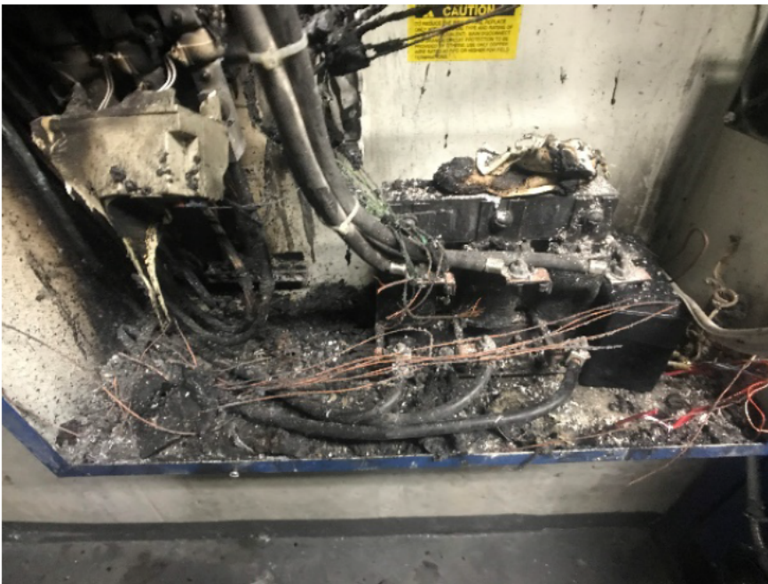
Photo 3 – Shows the fire damage just below motor contactor
