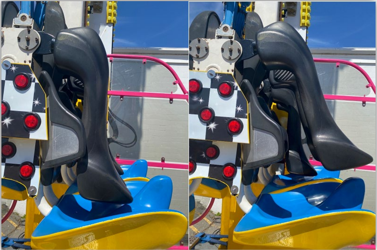
Photo 4 – Front rider seat, the restraint bar in the fully closed position (left) and the position locked by the secondary restraint mechanism (right).
