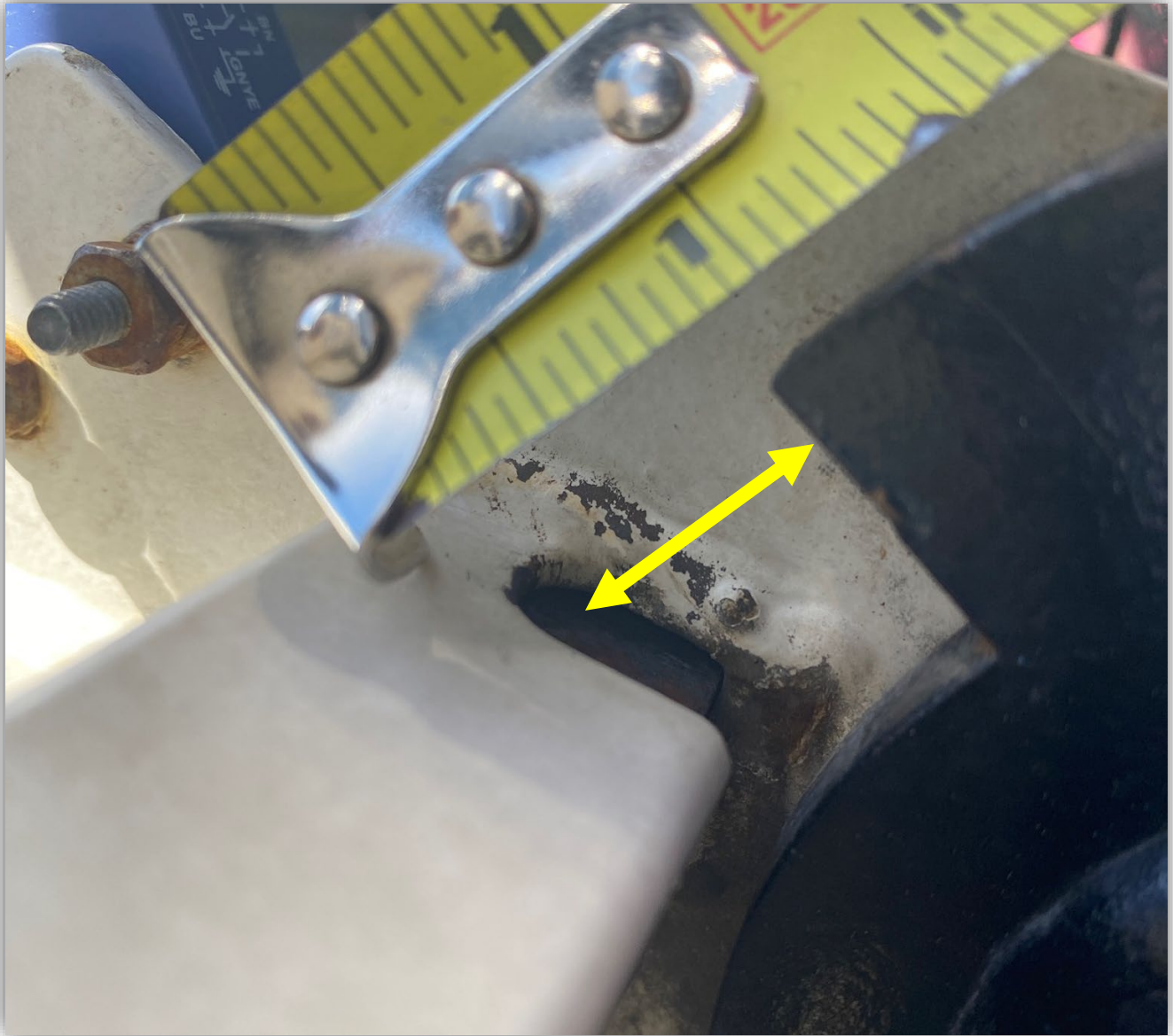
Photo 8 – Closeup of restraint bar cam and secondary locking bar. [YELLOW] Distance from cam to steel rod with the restraint in the fully closed position.
