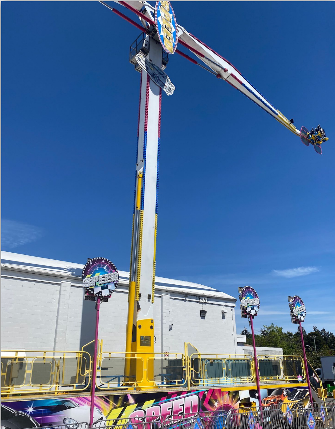
Photo 1 – Amusement ride set up - one side of the rotating arm with a 4-person rider gondola at the end.
