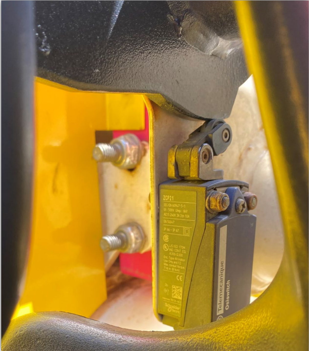
Photo 9 – Safety switch ensuring restraint bar is in the correct position to begin ride operation.
