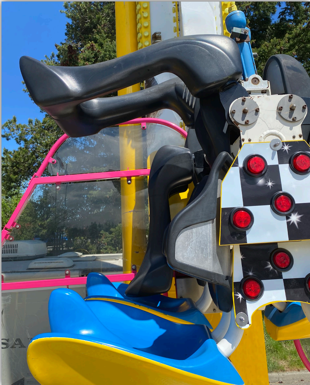
Photo 3 – Rider gondola - Restraint bars in the fully open (front) and fully closed (rear) positions.
