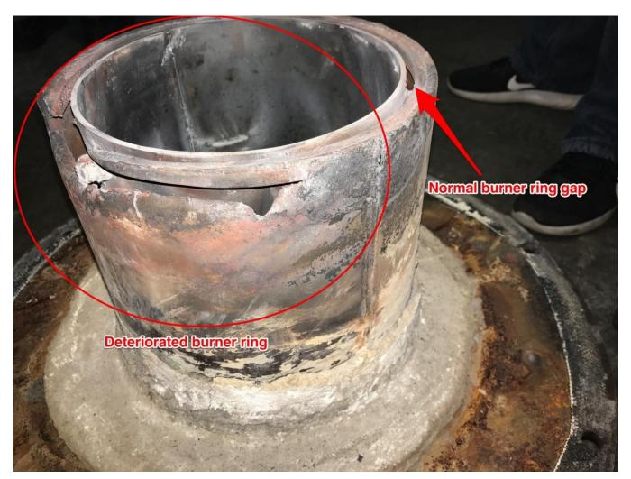
Image 11 - Burner housing with deteriorated ring and large gas port opening
