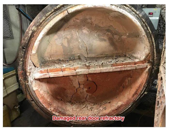
Image 8 - Cracked and broken rear door refractory insulation
