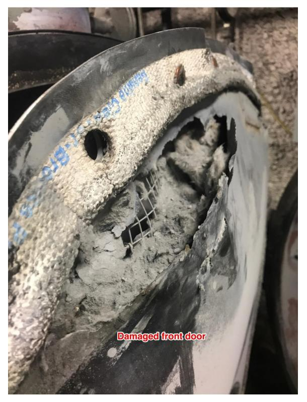
Image 7 - Damage to boiler front door
