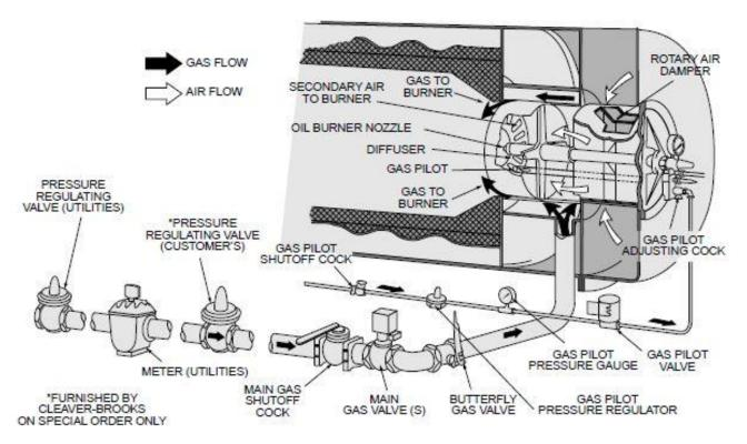
**Image 1 -** From the boiler manual, showing air and gas flow paths to boiler combustion chamber. The gas flows through the burner ring gap around the diffuser to mix with the air.
