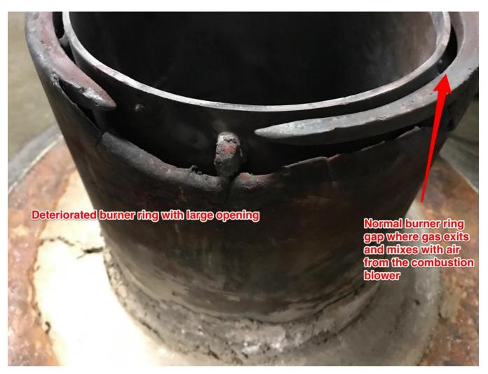
**Image 10 -** Burner housing with deteriorated ring and large gas port opening. The air diffuser gets positioned in the middle circular area of the burner housing.
