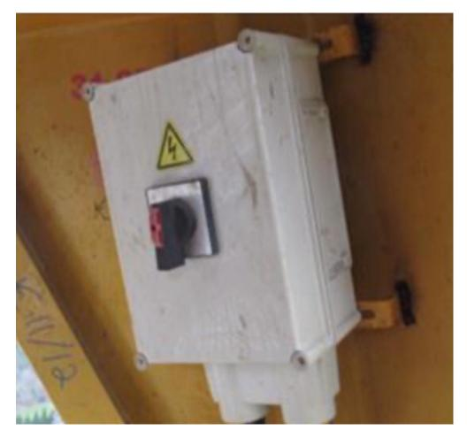
This photo is of the tower cranes manufactures disconnect switch located on the slewing ring level that turns power to the control panel where the incident occurred on and off.
