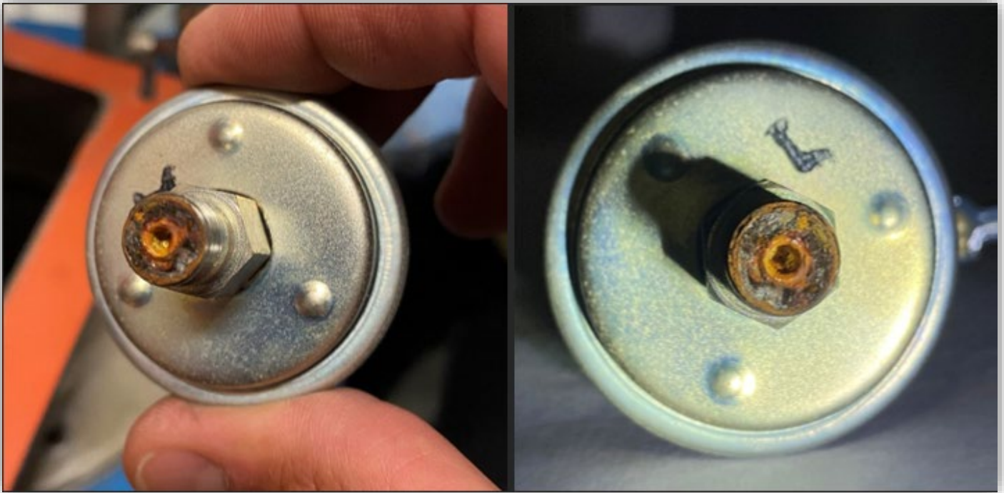
Image 11 – Corrosion plugged inlet to the high exhaust backpressure switch for Boiler #1.
