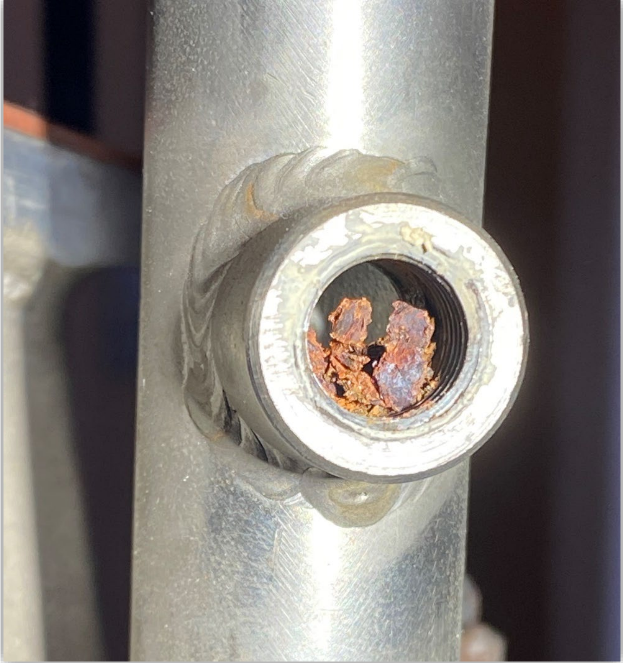
Image 9 – Corrosion debris inside 1/4" outlet housing the black iron street elbow for the high exhaust backpressure switch.
