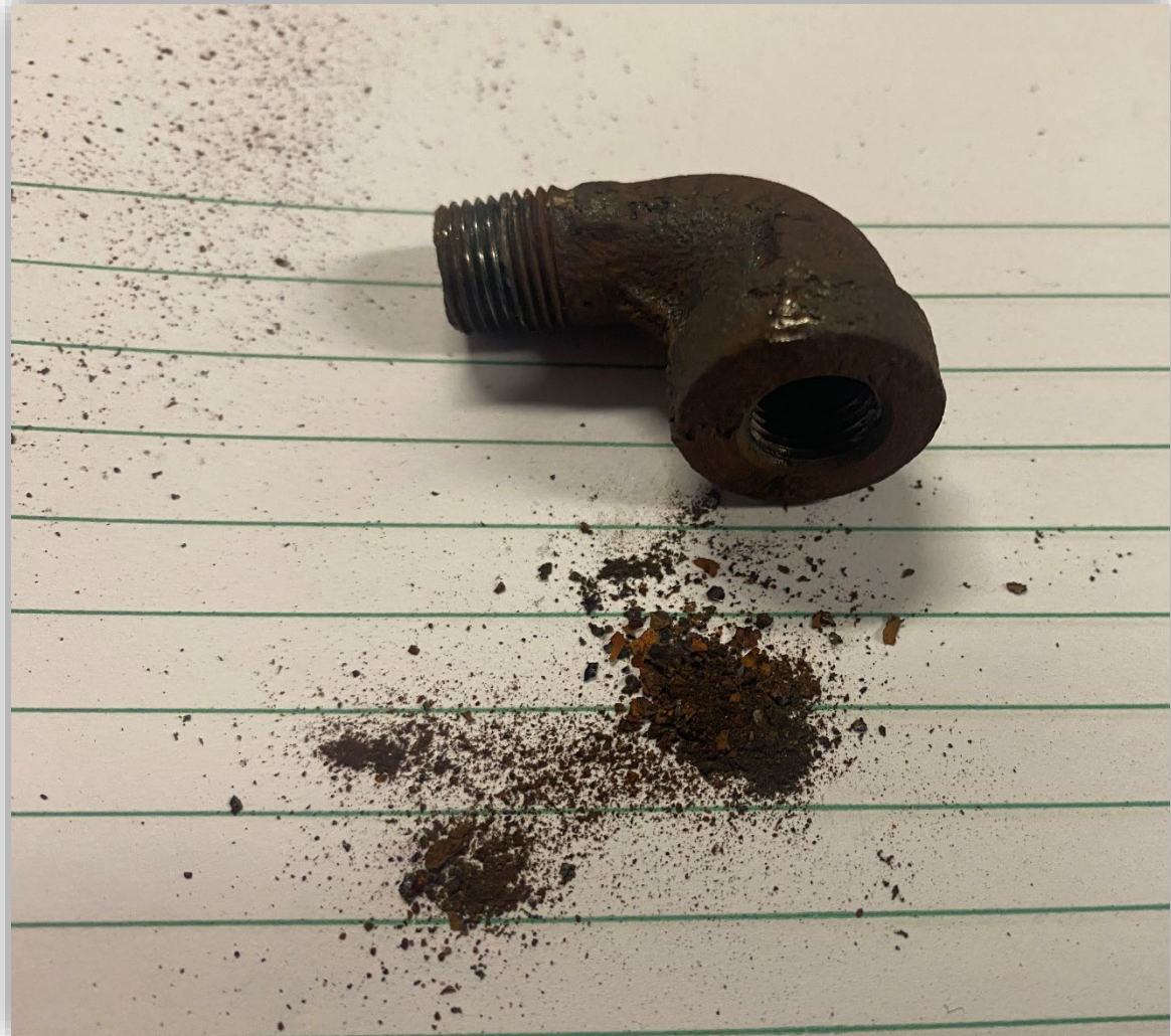
Image 10 – Corrosion debris from inside black iron street elbow housing the high exhaust backpressure switch.
