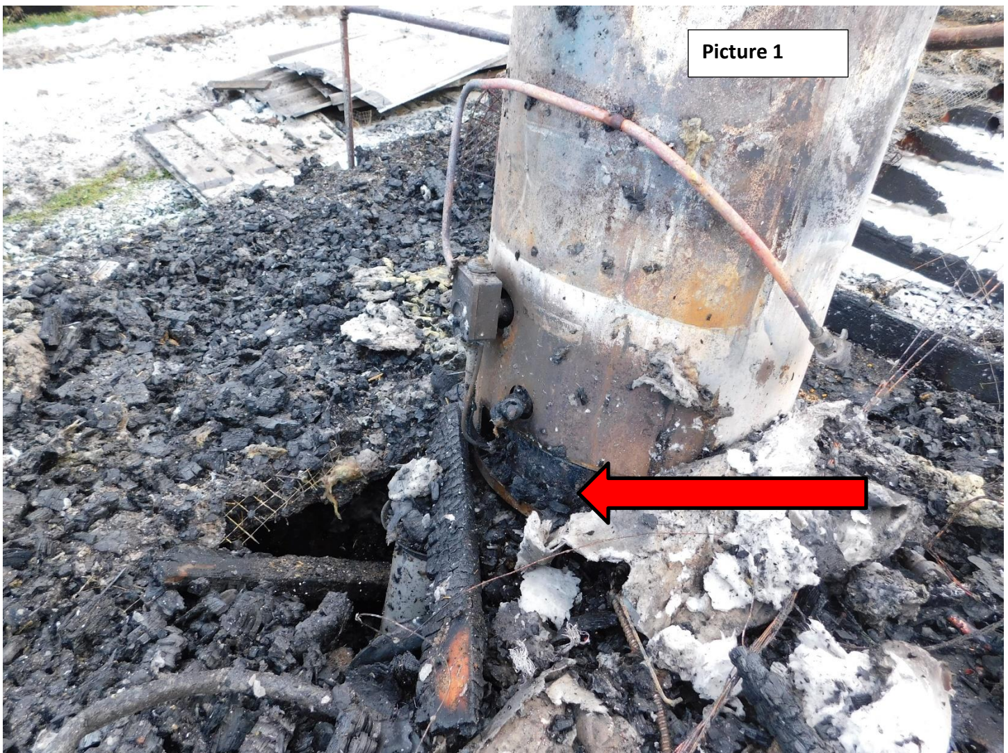
Water heater found in the barn that was destroyed. Burner compartment was closely examined and found to have a large accumulation of organic materials within. (Red arrow points toward burner compartment)
