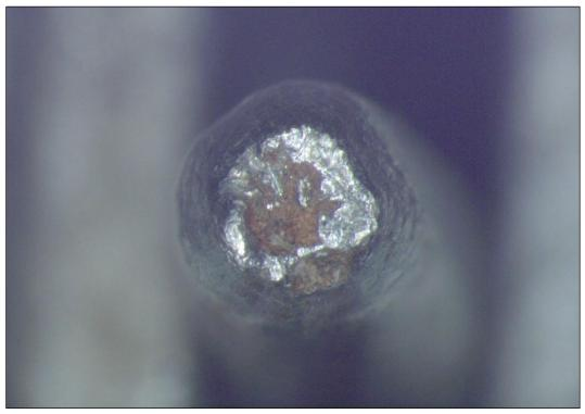
Figure 13 Cup and cone tensile overload on strand 2. Outside wire 10.
