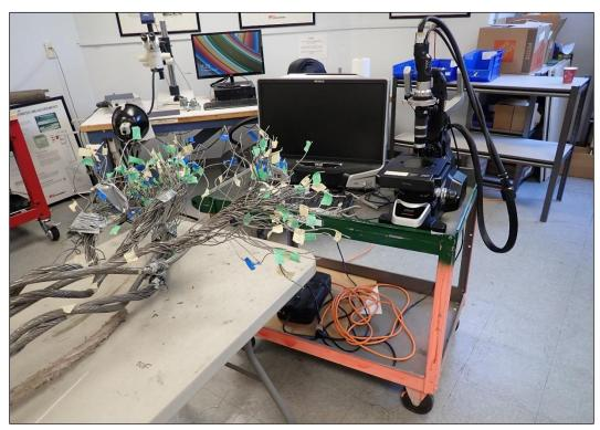
**Figure 6** Fractured wire ends labelled with yellow, green and blue tape corresponding to labels used in Tables 1 – 6 (Appendix B) describing fractures. Keyence microscope used to magnify and document end features is shown in background.
