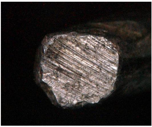
Figure 9 Typical through -cut wire on strand 3. Outside wire 7.
