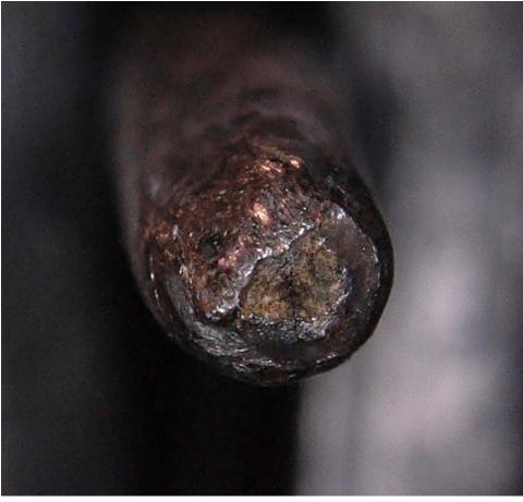
**Figure 12** Cup and cone tensile overload on strand 1. Outside wire 13.
