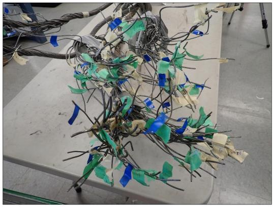
Figure 7 Closer view of wire ends on downhill side of severed haul rope.
