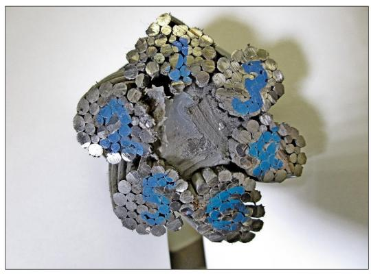
**Figure 5** End of haul rope as cut at site. Strand are arbitrarily labelled 1 – 6.
