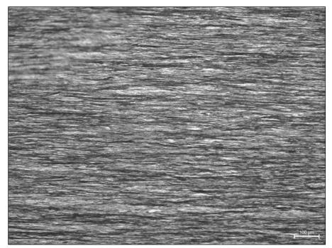
**Figure 14** Typical wire microstructure. Microstructure is severely cold worked ferrite-pearlite. Sample has hardness of HVN 262 (etched 2% Nital; Mag. 200X).
