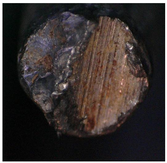
Figure 11Partially cut wire on strand 3. Outside wire 2.
