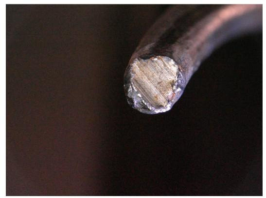
**Figure 10** Partially cut wire on strand 4. Outside wire 6.
