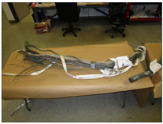
Figure 1Uphill end of severed haul rope.
