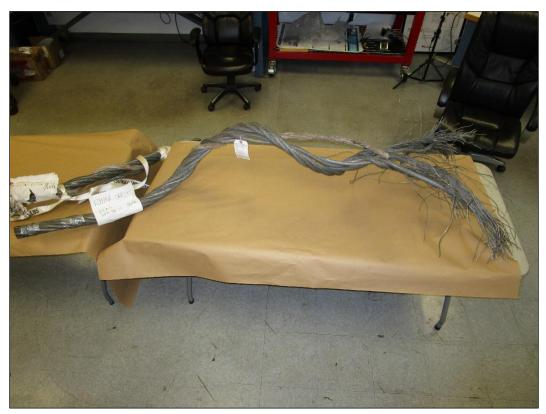
**Figure 2** Downhill end of severed haul rope.
