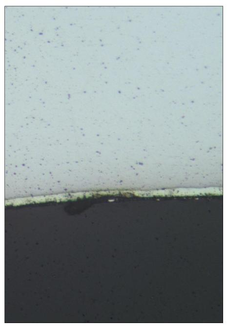
**Figure 15** Typical galvanizing layer on wire strand. Zinc layer is uniform and approximately 10 microns thick. (mag x 200; Unetched)
