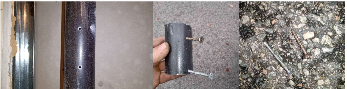
Figure 2 - Gas pipe with holes (left), screws in the pipe (center) and after removal (right) One of the self tapping screws was likely replaced with a wood screw during install.
