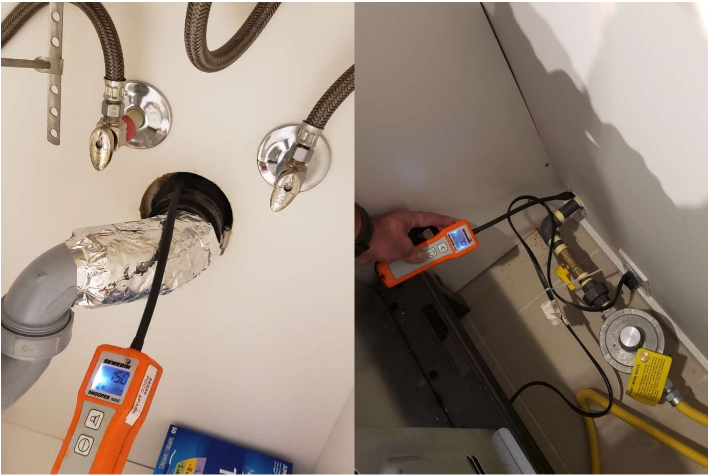
Figure 4 - Utility gas technician test results 150 parts per million (ppm) under bathroom sink (left) and 70 ppm behind kitchen stove (right)
