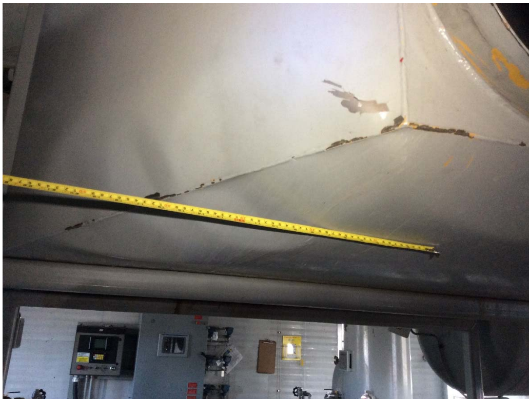
K-440 rear damaged intake as observed – note intake bulged
