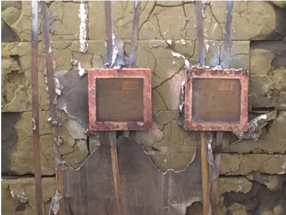
V-665 Low Temperature Separator – Nameplates damaged by fire.
