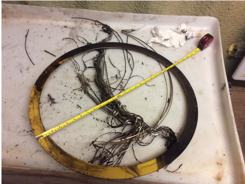
V-665 Low Temperature 18 Inch Inspection Nozzle gasket – removed by Owner representative
