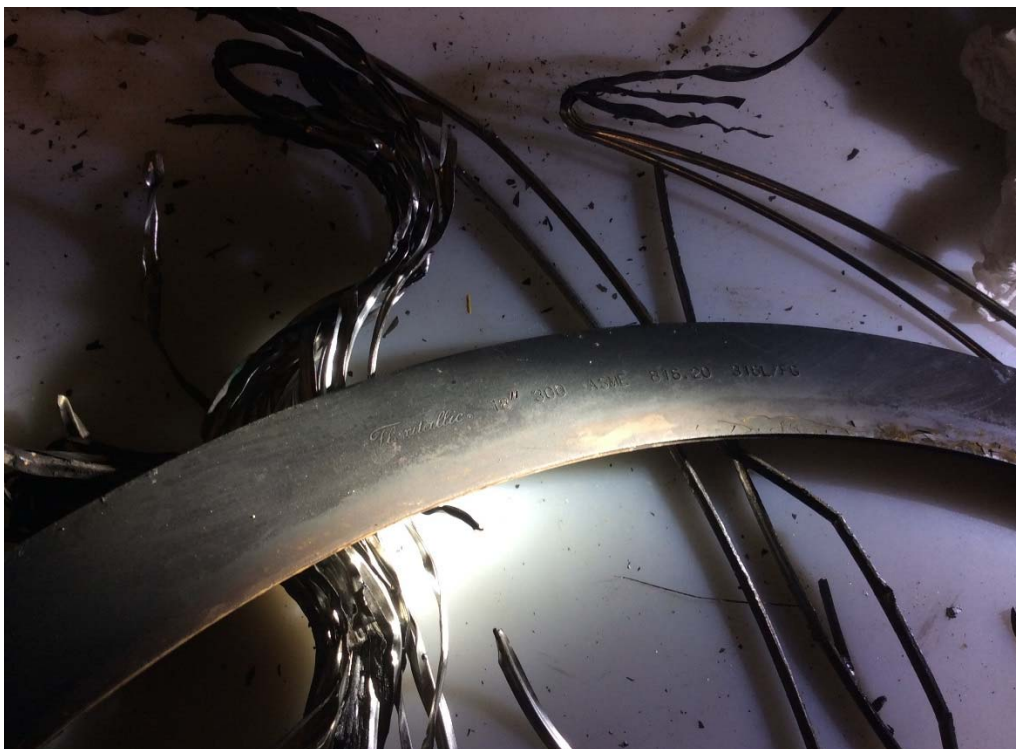
V-665 Low Temperature 18 inch Inspection Nozzle gasket – Note: rated only for 300 lbs class
