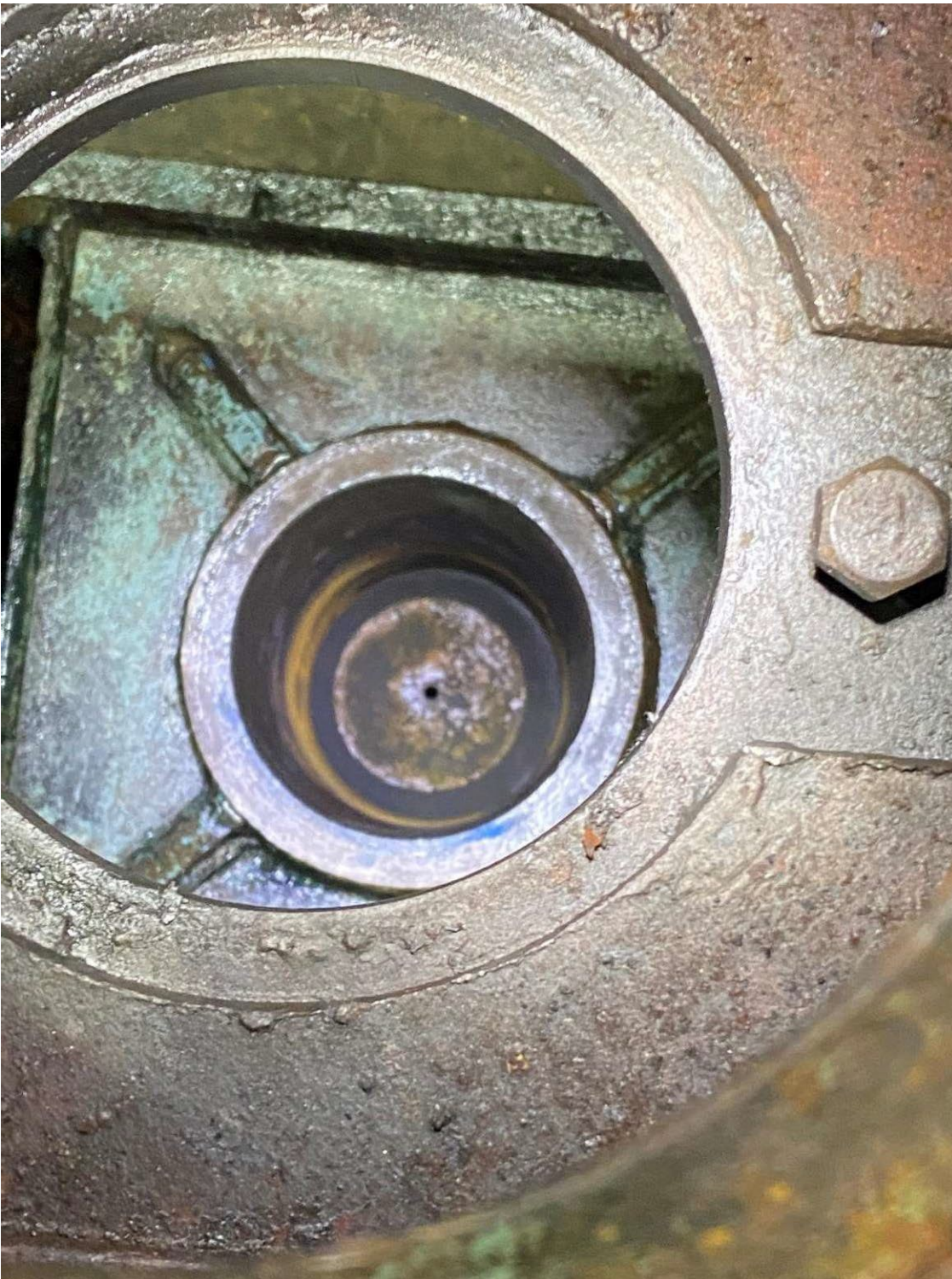
Photo 4, Photo of upper and lower bull wheel axle bore (axle and sleeve removed). Looking through both the upper and lower horizontal hollow structure sections (*note, rust in lower bore) (**note, the small hole in the lower bore did not provide a drainage feature).
