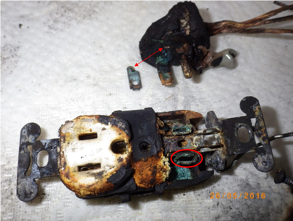
Figure 8 - Receptacle, cord end, and cord blade removed from the receptacle. Red arrow shows where the cord end blade was detached from the cord end. Red oval shows the receptacle opening where the blade was removed from.
