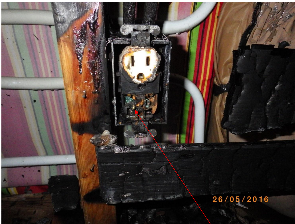
Figure 6 - receptacle with cord end removed. Cord end blade remained in the receptacle (red arrow).
