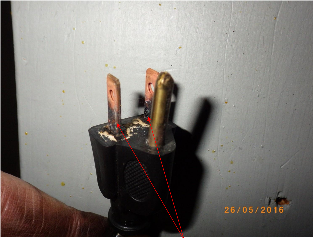
Figure 12 - One of the extension cords used in the bedroom shows signs of heat and discoloration on the cord end (red arrows). This was likely caused by over loading of the extension cord in the bedroom area. This example shows the improper use of extension cords in the bedroom area.
