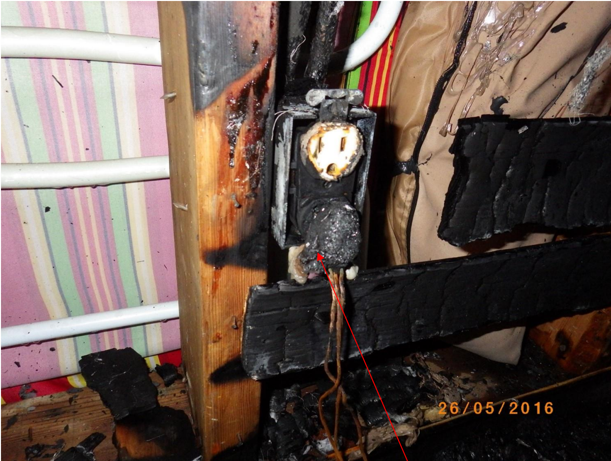
Figure 5 - bedroom receptacle with power bar cord plugged into the bottom outlet (red arrow). This is the point of origin.
