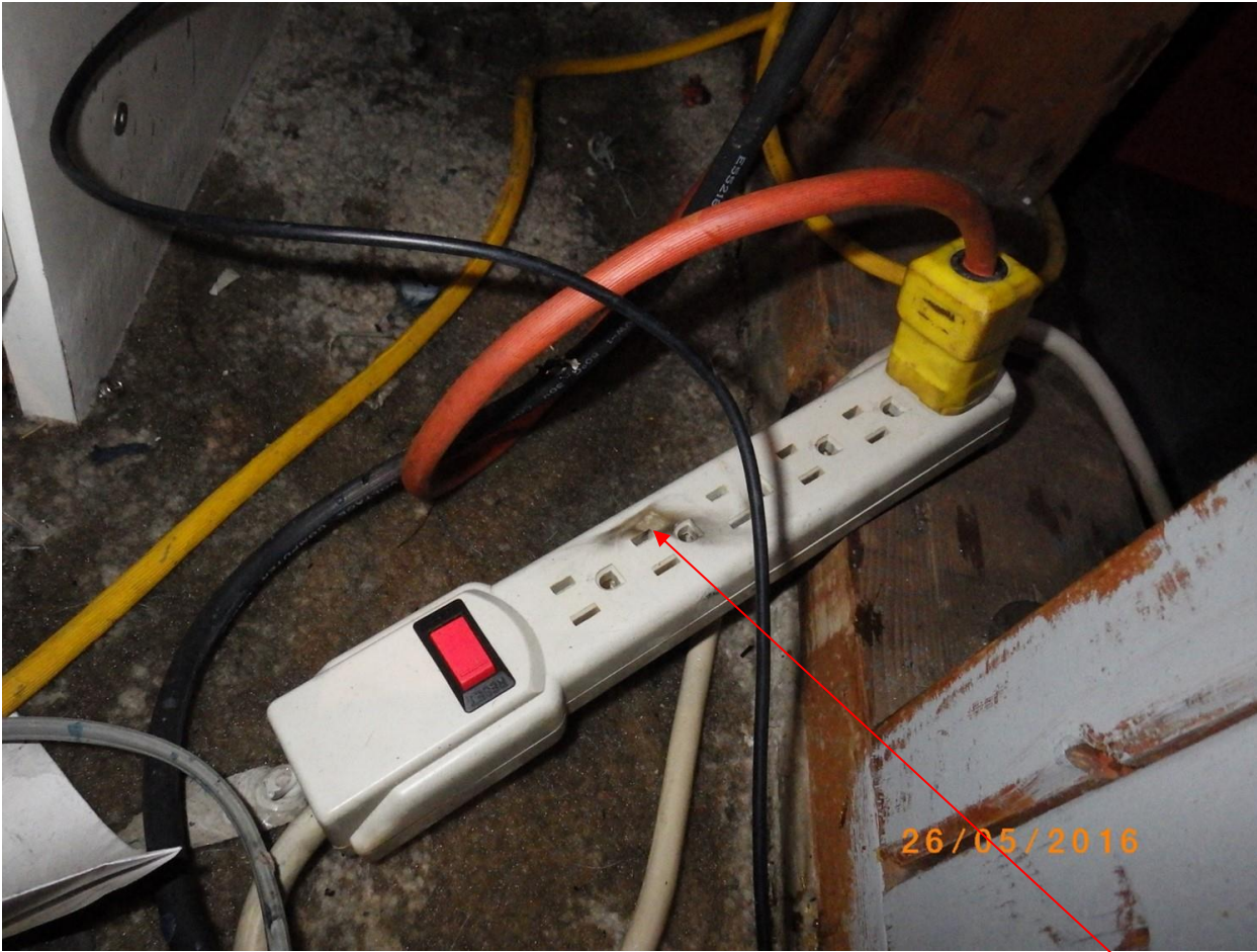
Figure 11 - One of the other power bars used in the bedroom shows signs of heat damage at one of the outlets (red arrow). This was likely caused by over loading of the power bar in the bedroom area. This example shows the improper use of power bars in the bedroom area.
