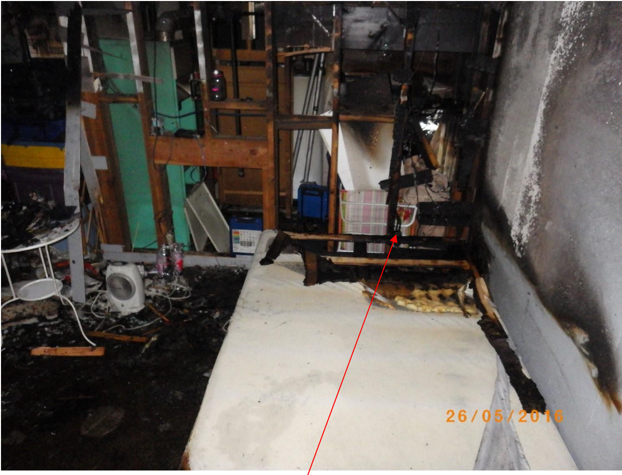
Figure 3 - Receptacle on the wall at the head of the bed where the fire originated (red arrow).
