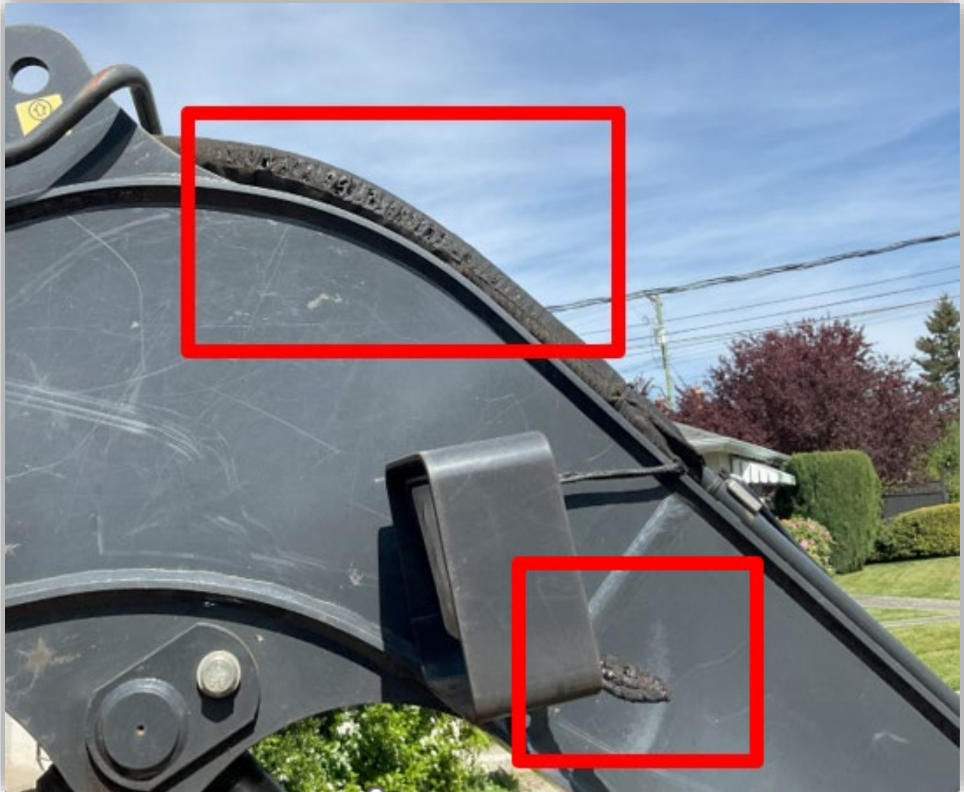
Image 5 – Excavator arm showing hydraulic and electrical lines damage from the fire.
