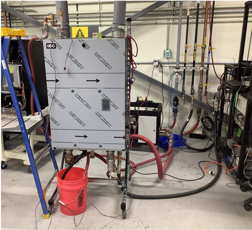
Image 2 – New boiler set up for testing in the manufacturer's laboratory.
