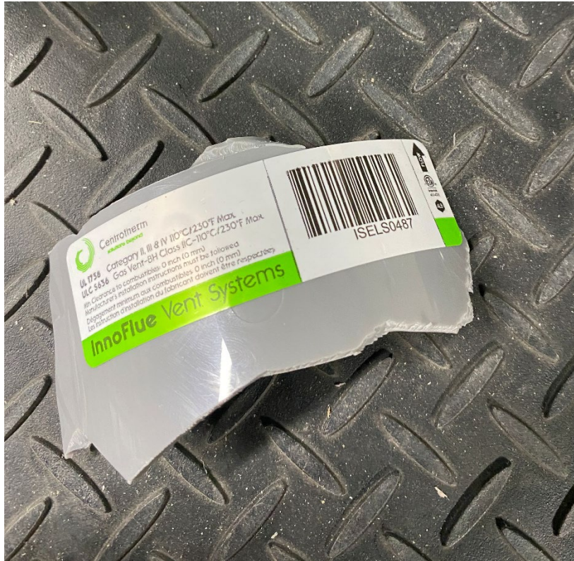
Image 9 – Broken piece of a vent elbow after it was propelled against the laboratory wall during a 2.5-second delayed ignition.
