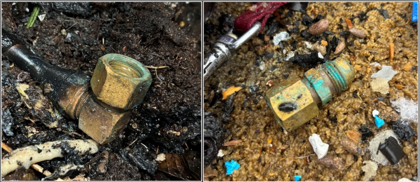
Image 10 – Closeup of unplugged gas line (Left) and gas line plug (Right) found in close proximity on the floor of the RV.
