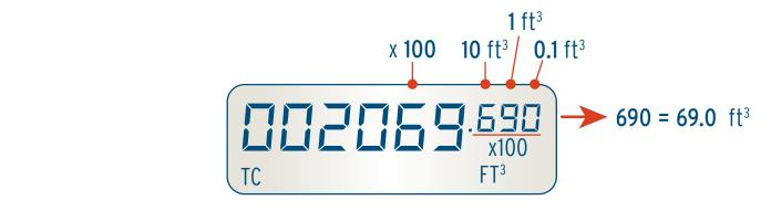
Note: Sonix IQ meters are only temperature compensated and will need the pressure correction factor applied when inlet pressure is greater than **0.5 psig**.
