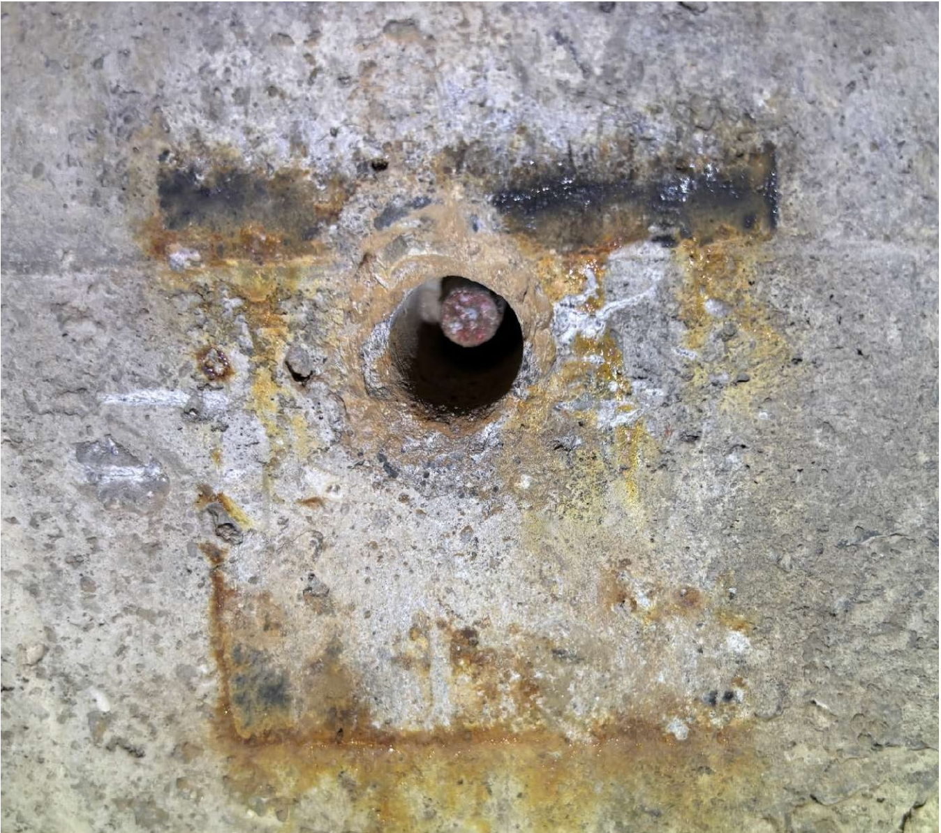
Image 8 – Concrete holed for failed anchor. Anchor set pin shown still attached to the center of the hole.
