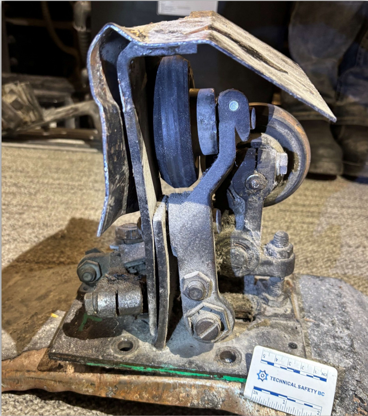
Image 12 – Second view of the damaged counterweight guide assembly.
