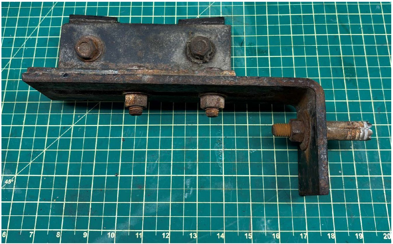
Image 16 – Counterweight guide rail bracket with concrete anchor still attached.
