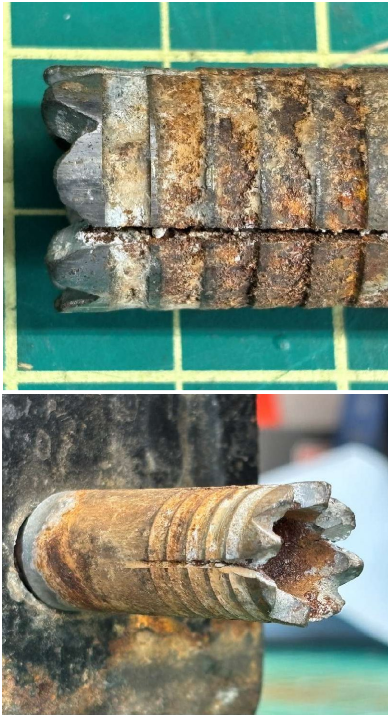
Image 17 – Closeup images of the failed concrete anchor.
