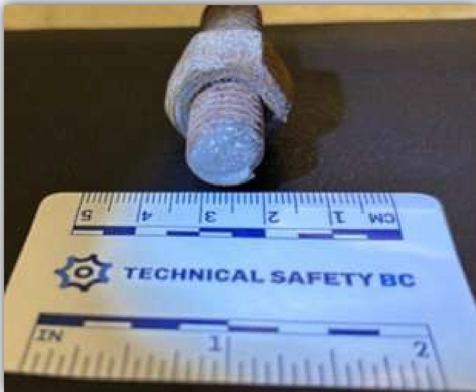
Image 10 – The other half of the broken threaded rod recovered from the elevator pit after the incident.
