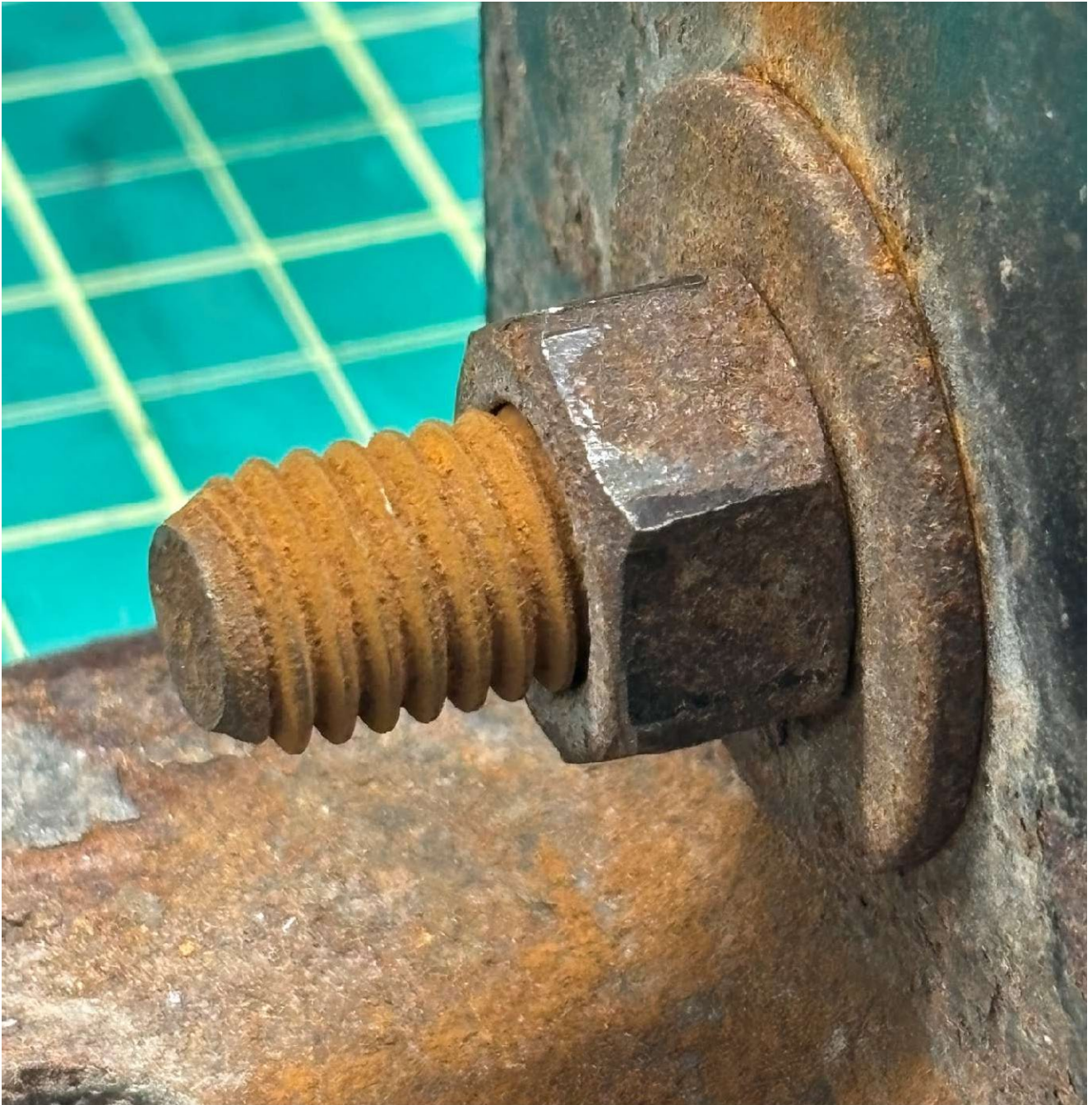
Image 18 – Closeup of threader rod, nut and washer still tight to bracket after concrete insert failure.
