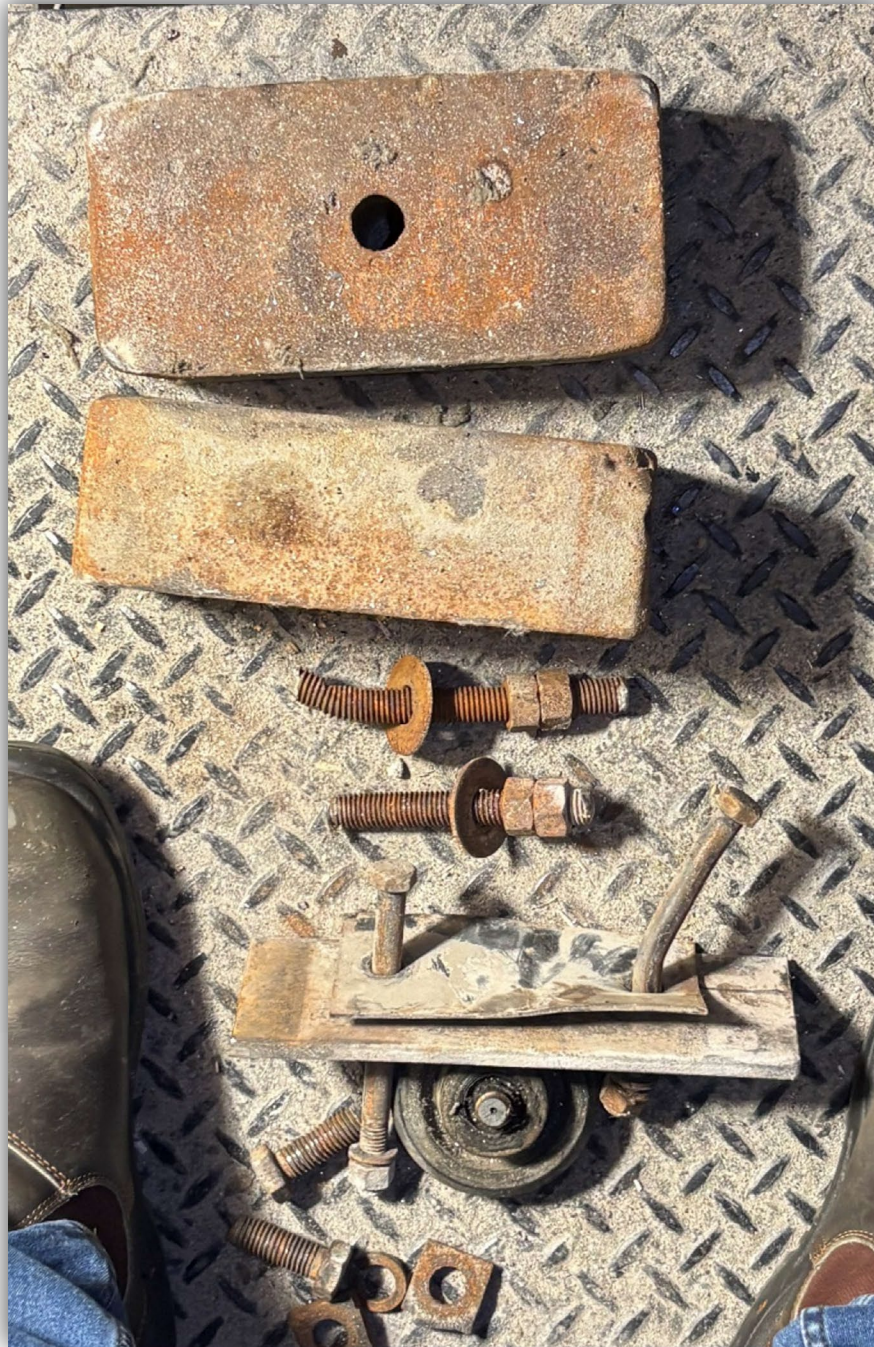
Image 14 – The two 50lb balance weights and damaged hardware that were torn from the bottom of the passenger car and crashed into the bottom of the elevator pit from the 17 th floor.
