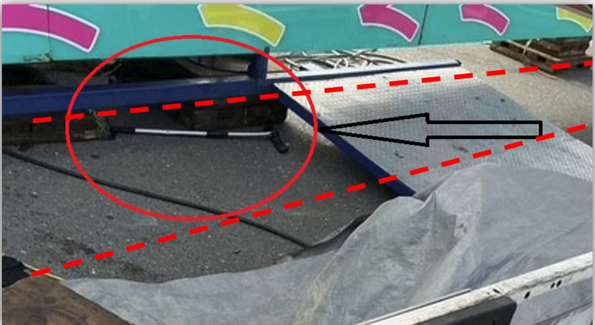
Image 6b – After incident magnetic broom found under ride path zone.
