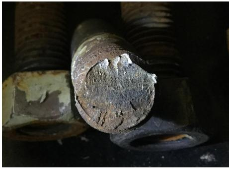
Figure 4: Fracture face of stud #1
