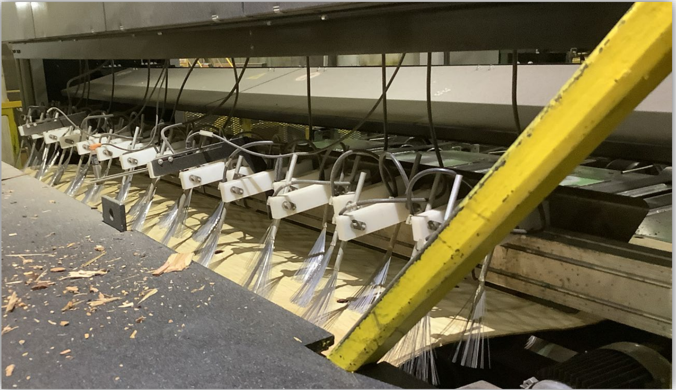
Image 5 - Sensing brushes below with 7Vac sensing circuits measuring moisture in sheets as they cross the brushes to 0-volt sensing brushes.
