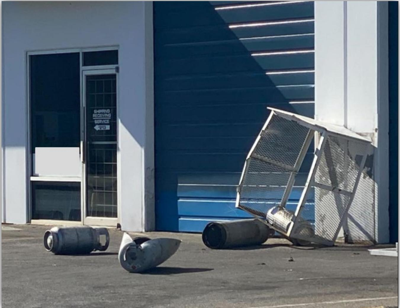
Image 3 – Damaged cylinders and cabinet.
