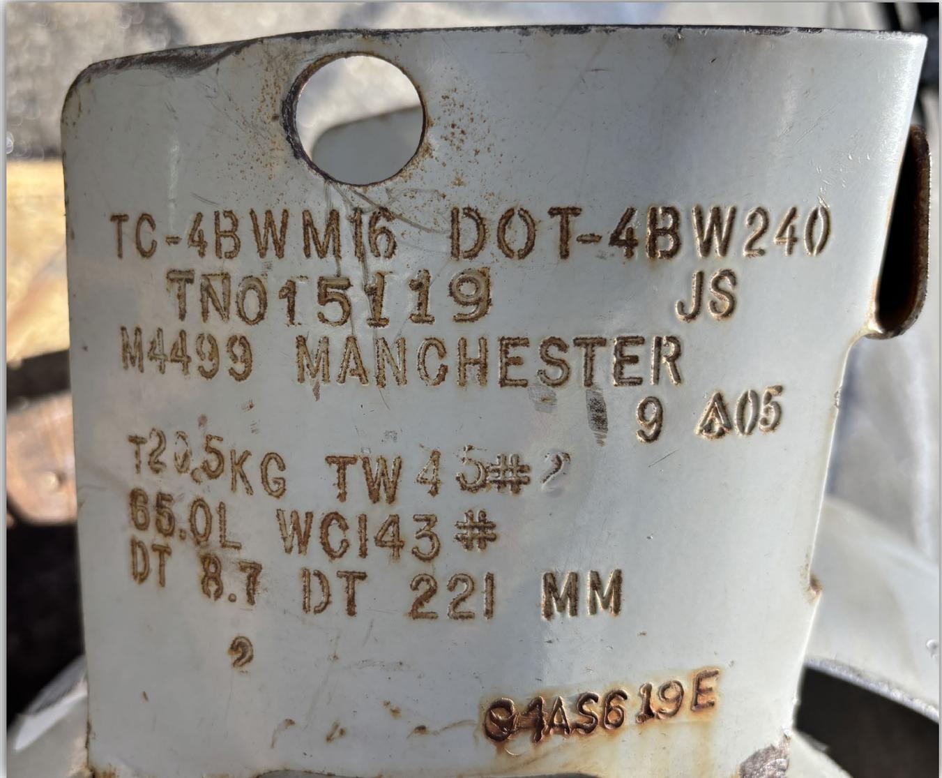
Image 6 – Cylinder collar showing original manufacture date, tare weight, water capacity, dip tube length and the recertification date of 04, 2019 and the recertification facilities Transport Canada code.
