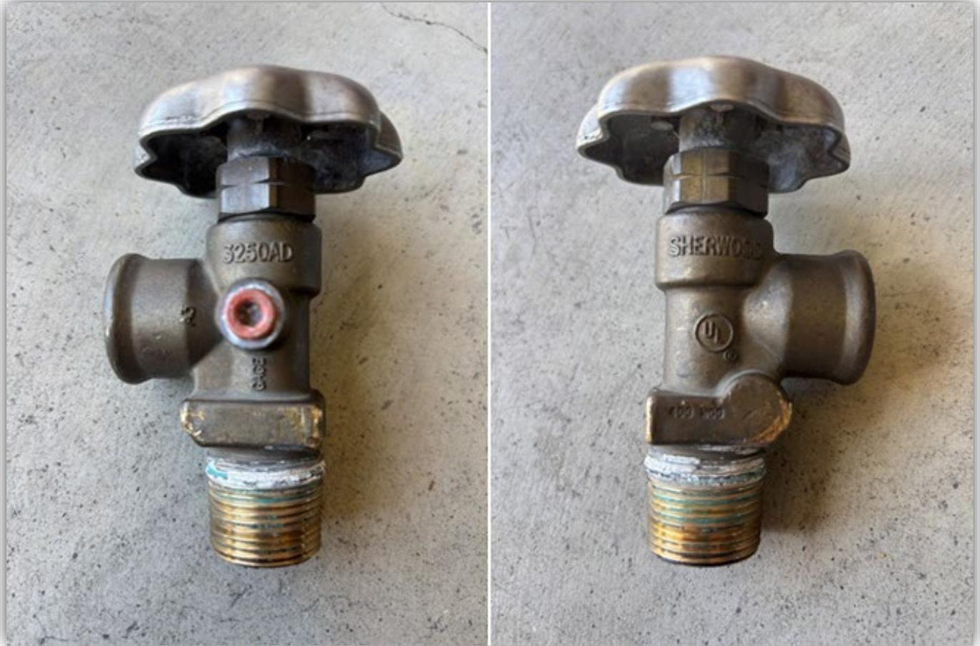
Image 7 – Sherwood 3250AD service valve removed from damaged cylinder without a dip tube or relief valve.
