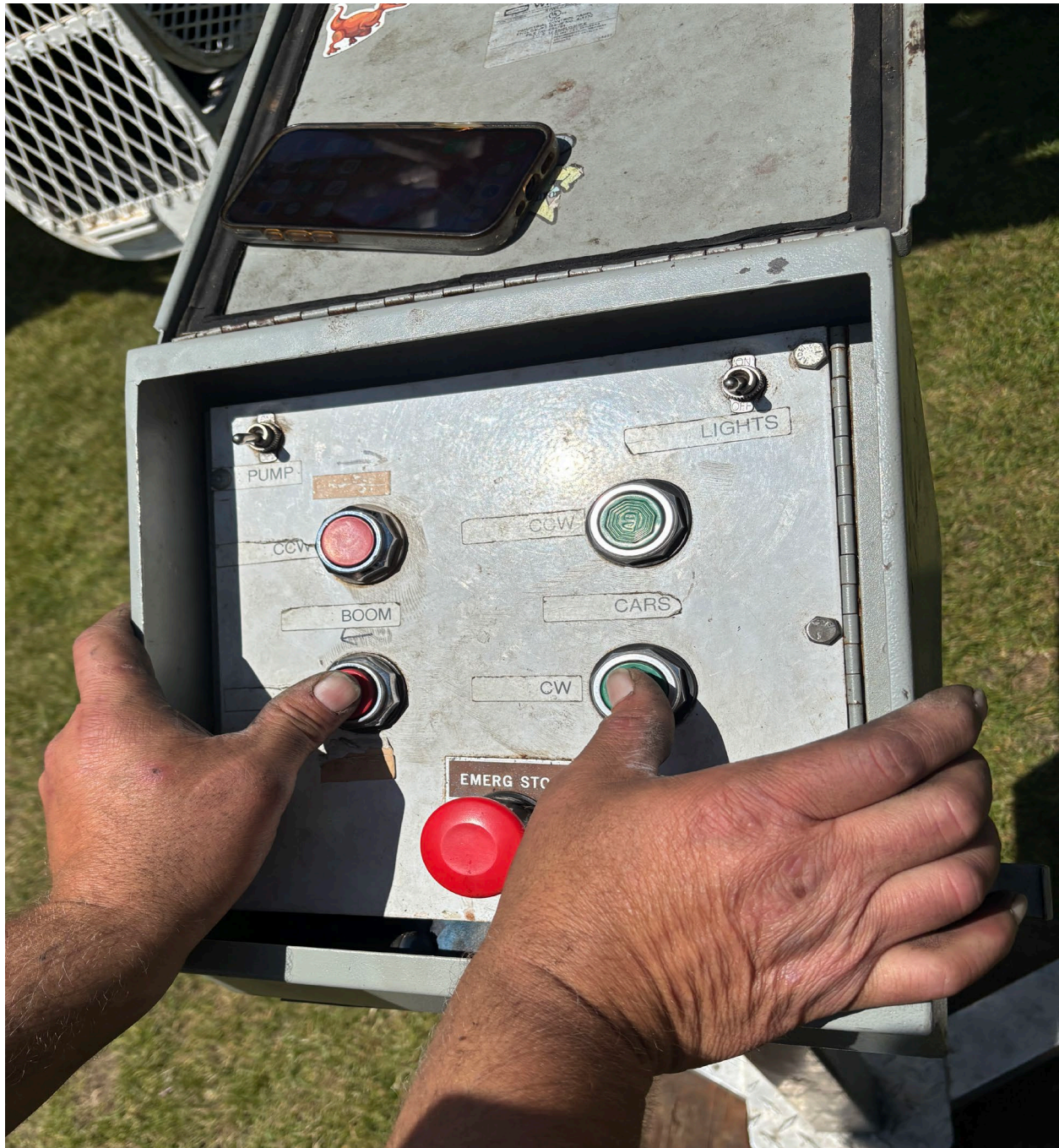
Image 5 - Ride operator controls showing typical hand position of the operator on the start and stop buttons for loading and unloading.
