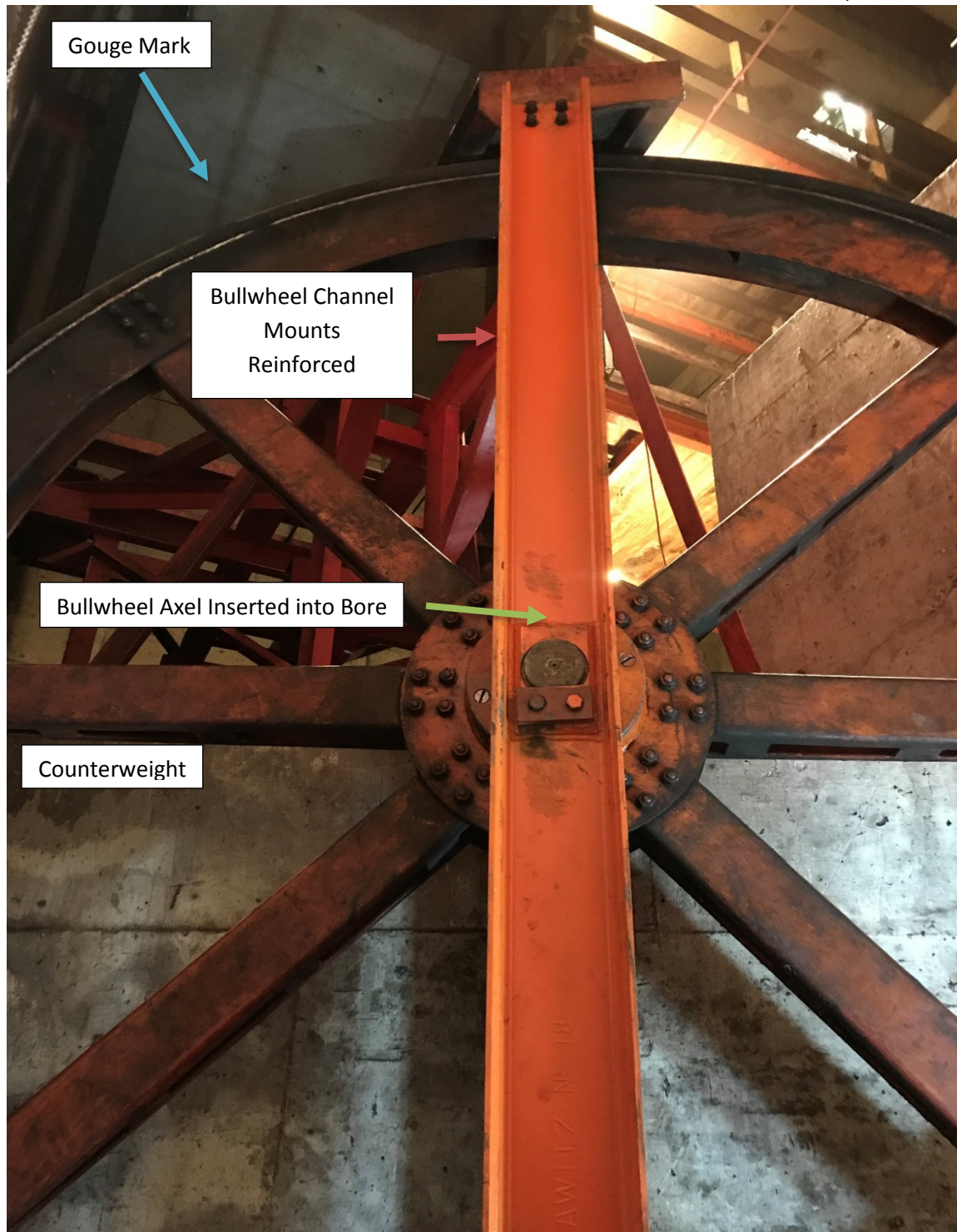
Figure 3, Photo of Gouge Mark in Outer Diameter of the Counterweight Bullwheel. (Photo taken after due to the incident extra reinforcement had been added to channel mounts)
