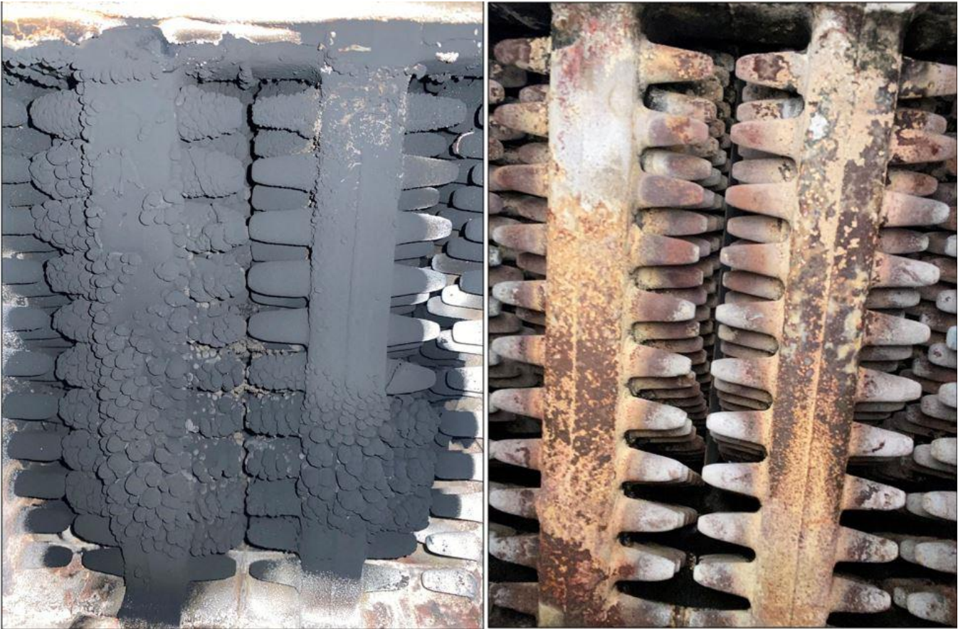
Image 6 – Soot and carbon deposits found on the boiler heat exchanger following the incident (left) and after cleaning (right). The soot and carbon deposits restricted the flue gas passage through the heat exchanger.
