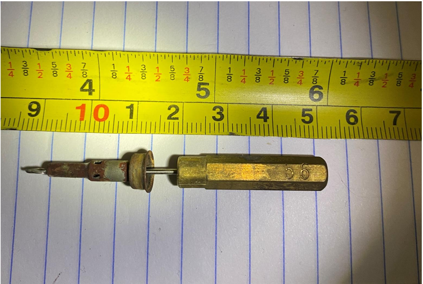
Image 9 – Pilot orifice with a #56 orifice drill (0.0465") inserted to measure the size of the enlarged gas flow opening
