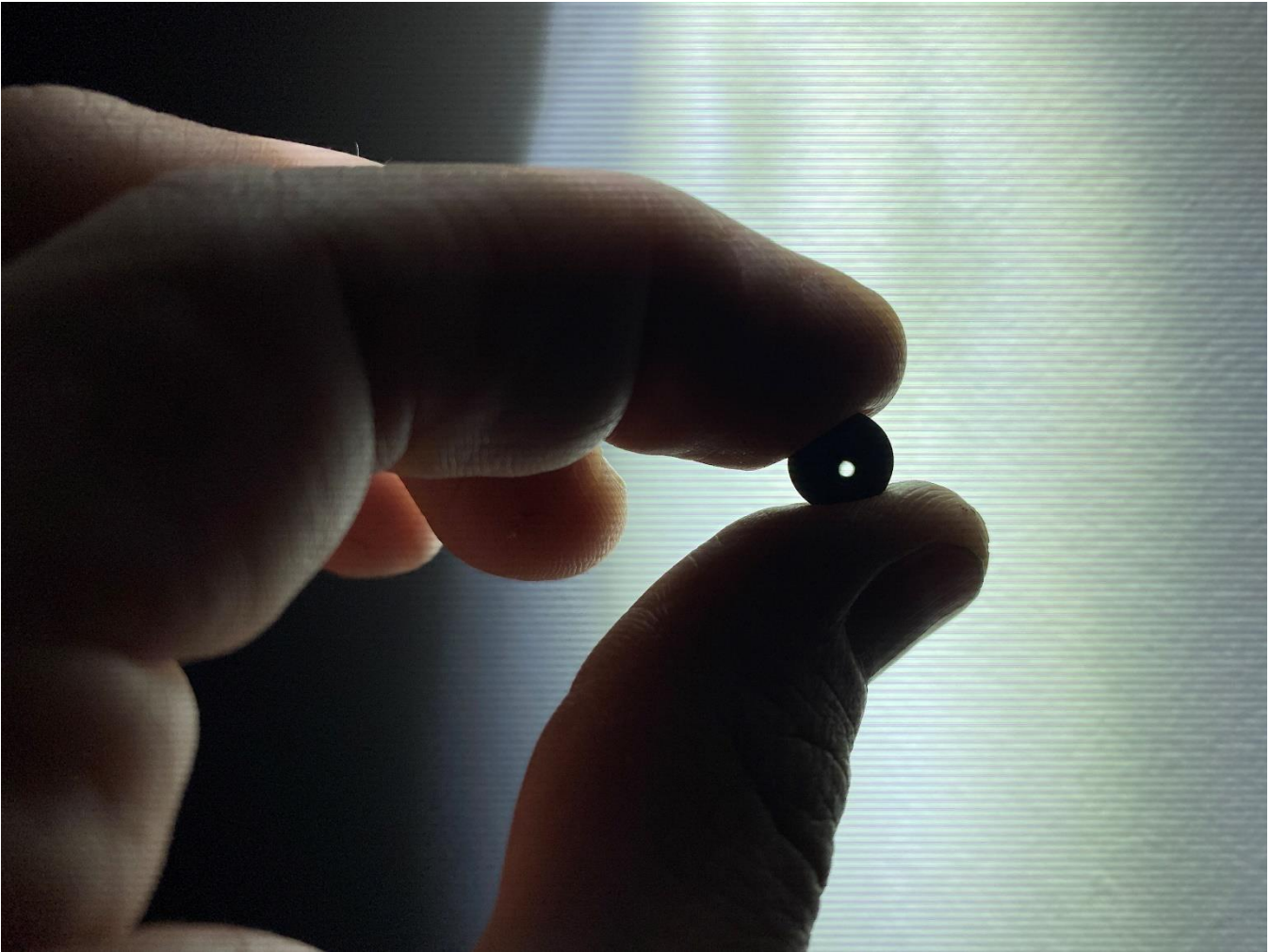
Image 8 – Pilot orifice showing the enlarged size of the gas flow opening
