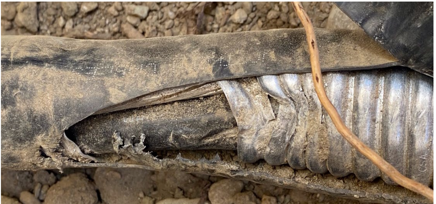
Photo 6 - Damage to outer jacket and armour of cable where bucket came in contact with cable.
