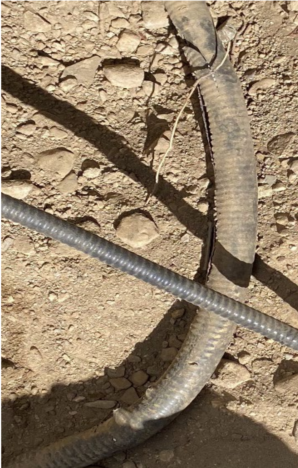
Photo 4 - Damage to outer jacket of cable where bucket came in contact with cable.
