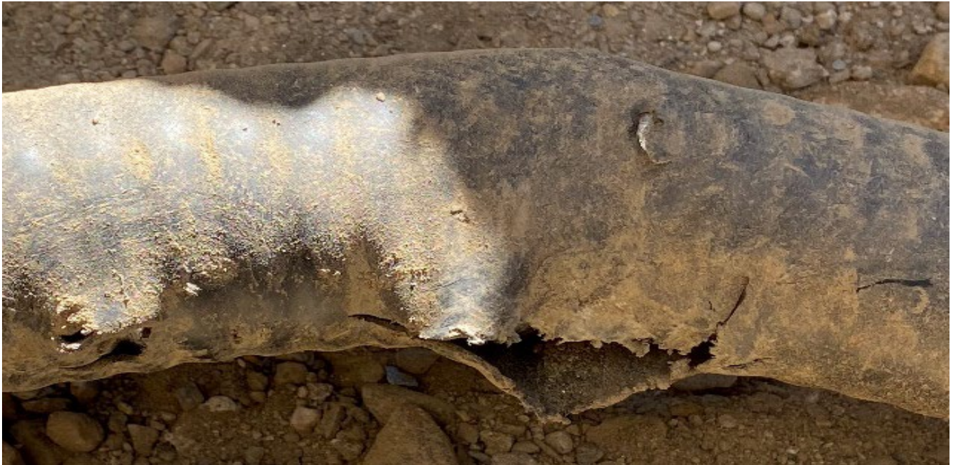
Photo 5 - Damage to outer jacket of cable where bucket came in contact with cable.
