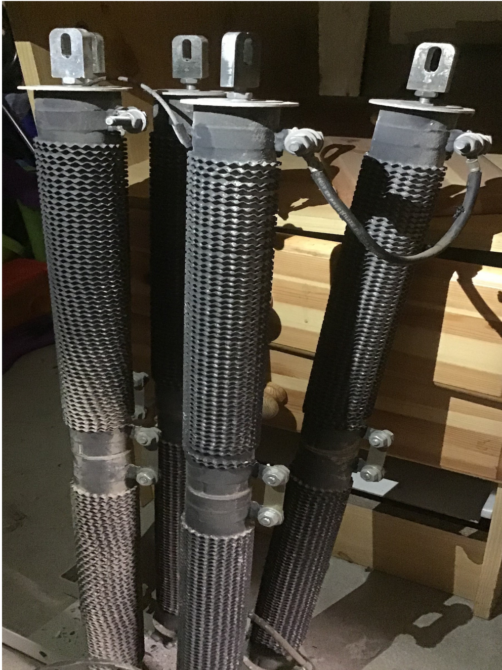
Photo 2: The original braking resistors that were replaced after being affected by the transistor failure.
