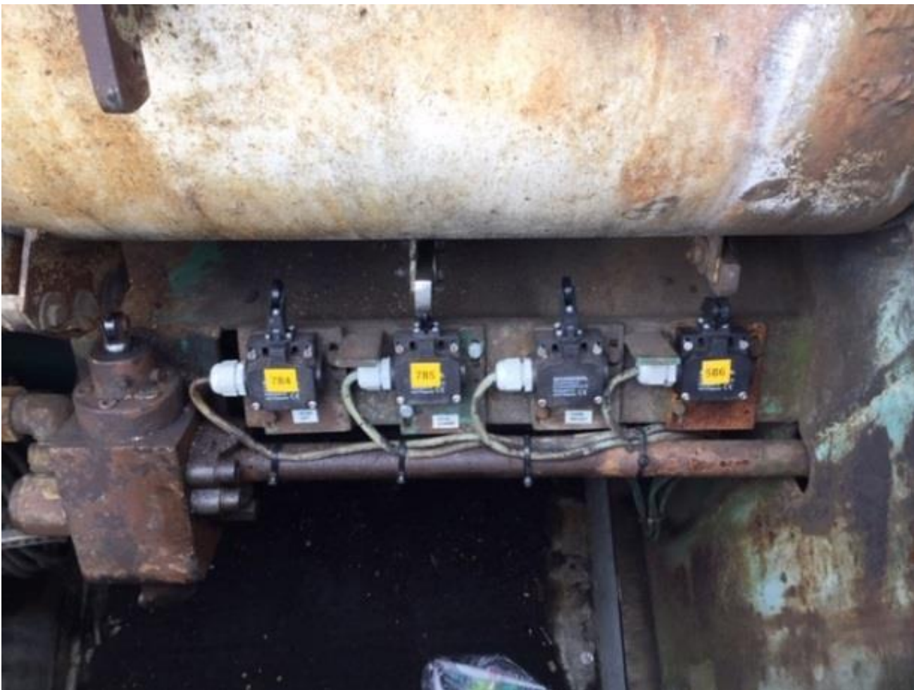
Proximity switch rack, and base of hydraulic arm with actuator cam(s)
