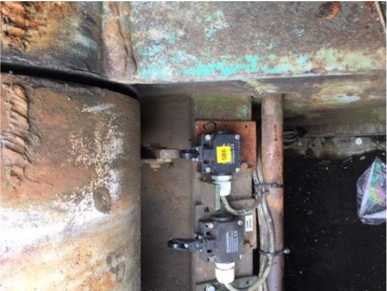
Proximity switch 5B6, proximity switch bolted mounting plate, hydraulic arm actuator cam.
