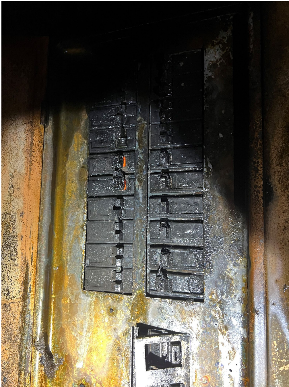
Image 7 - Front view of panel in place. No openings noted, no evidence of fault/flames exiting front of panel.
