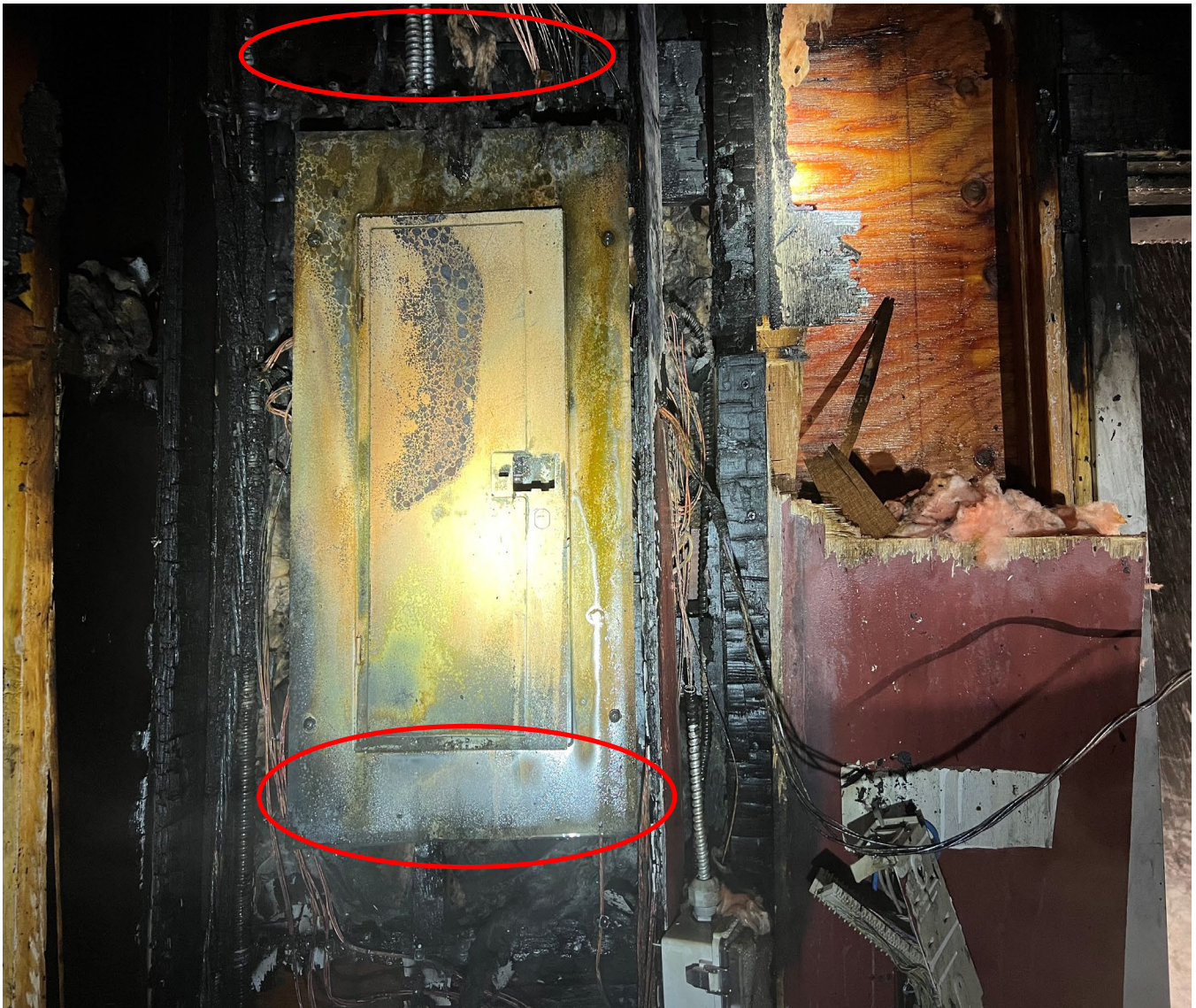
Image 1 - Fire damage above and below the electrical panel and contained in the stud space of panel and cables
