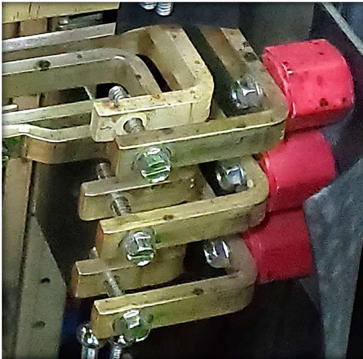
Figure 6 (bottom) – General area of arc flash showing damage to and travel of bus bar jumpers (arrow), and burn marks from arc flash
