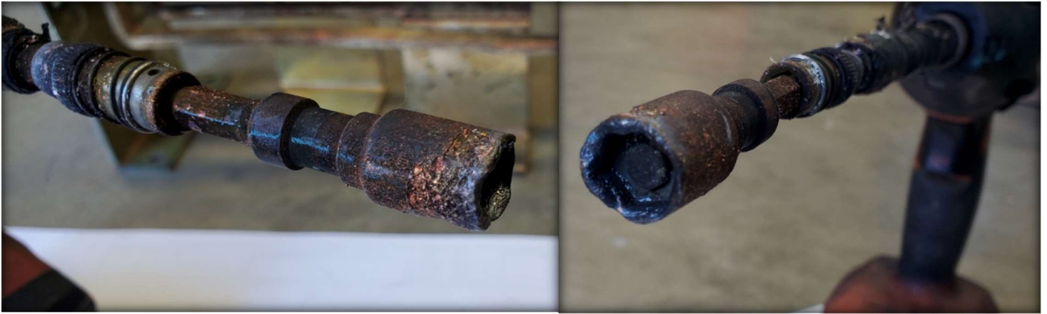
Figure 9 a, b - Nut driver end melted on the side and at the end from arcing to energized component(s)
