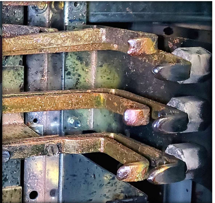
Figure 6 (bottom) – General area of arc flash showing damage to and travel of bus bar jumpers (arrow), and burn marks from arc flash
