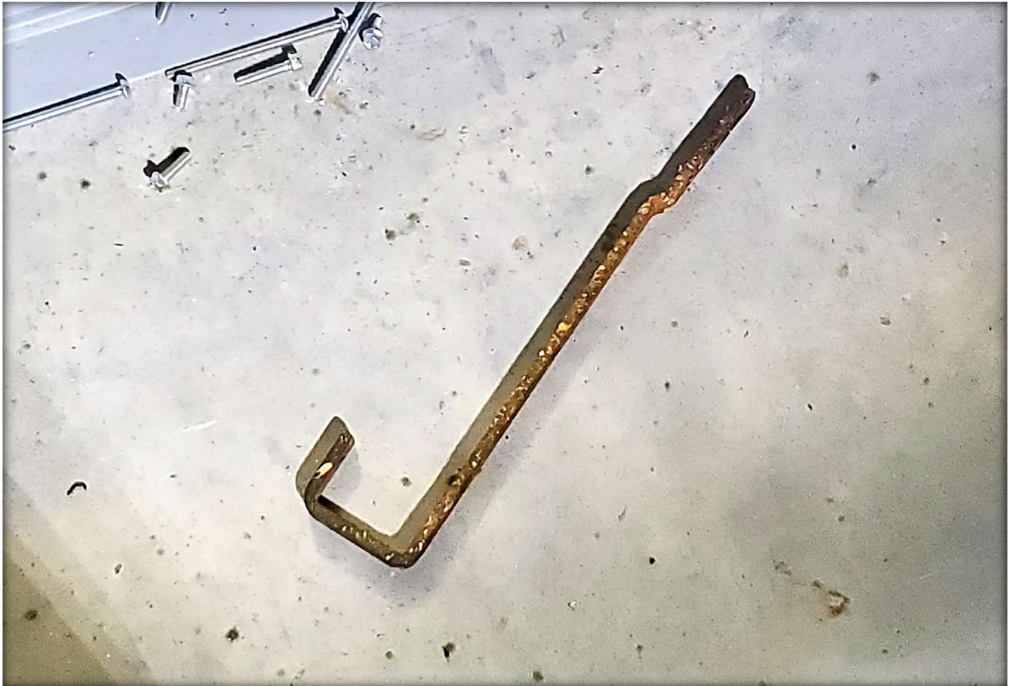
Figure 10 - Bus bar jumper showing signs of melting damage on the floor in front of the MDC
