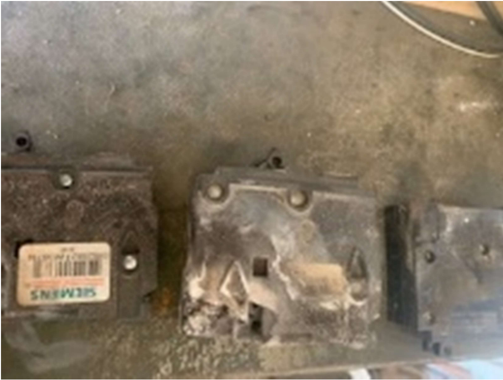
Image 4 -Siemens label on breaker installed to Homeline panel
