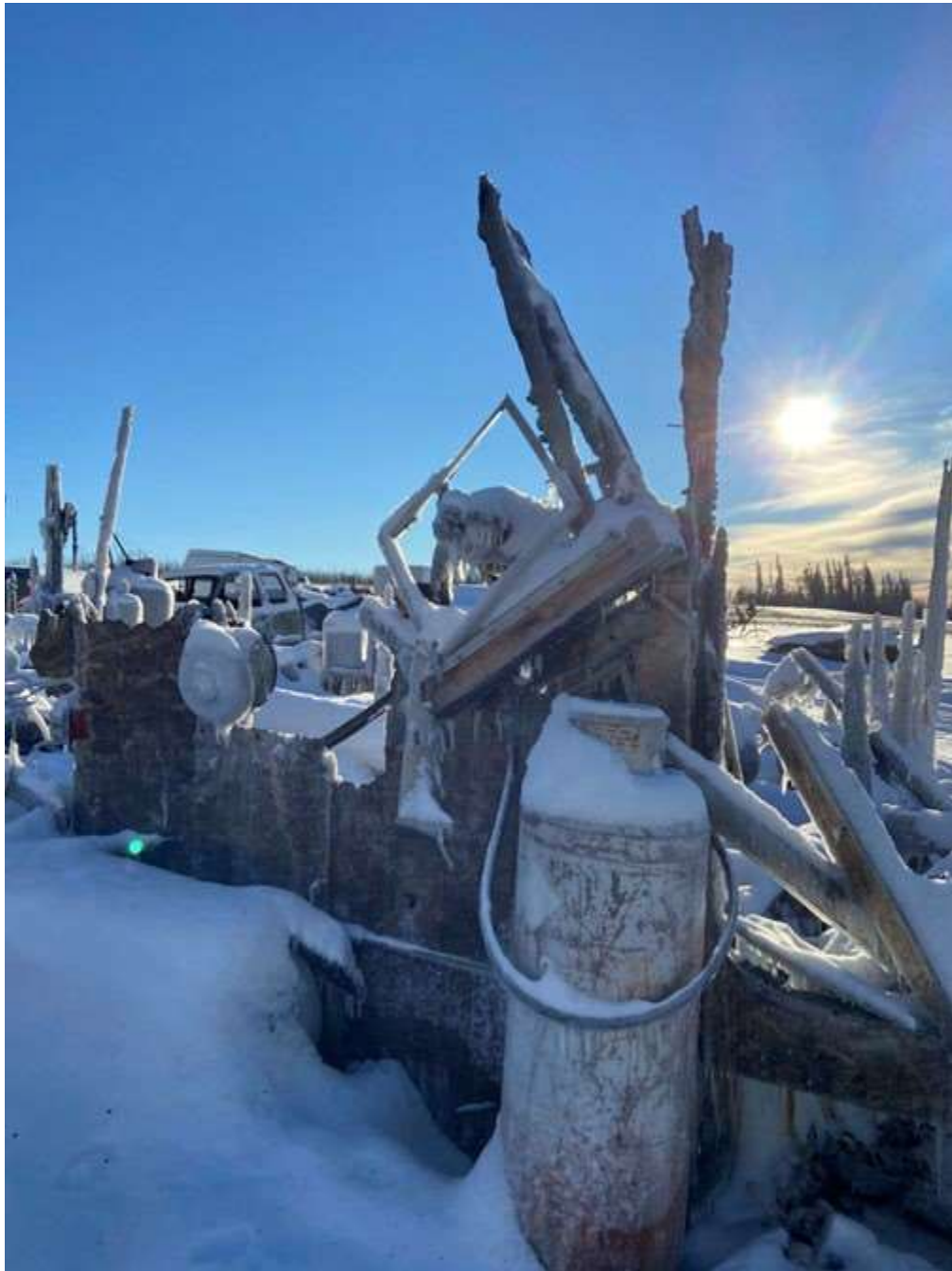
Photo 3 – 100-pound propane cylinder outside the residence connected to an RV style appliance.
