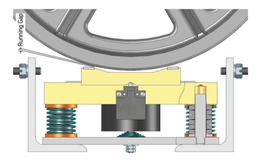
2) The device should be kept clean [especially the following areas frictional plate teeth (Y), Bearing plate (B)]; do not allow a build-up of foreign material to occur, as this can undermine the device's ability to function properly.
