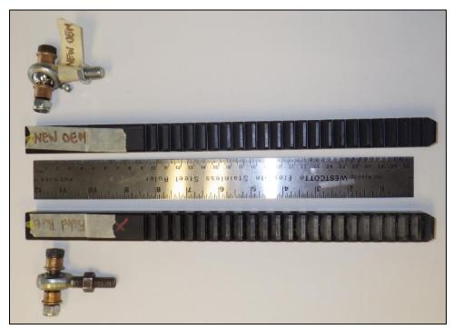
Figure 2: Trunnion bolts and ratchet shafts, incident (below) and new OEM samples (above).
