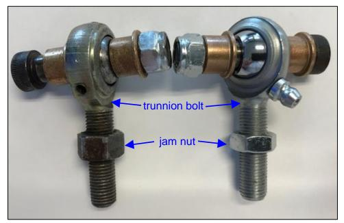
Figure 1: Incident trunnion bolt (left) compared to new part from the original manufacturer (right)
