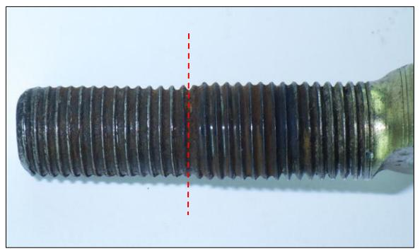
Figure 5: Bolt threads heavily worn, narrowing the bolt diameter below nut position (left of red line)
