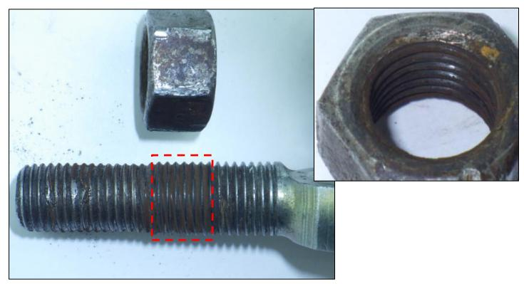
Figure 4: Nut removed showing rust on bolt and nut threads were they were seized together.
