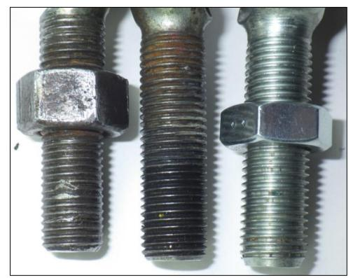
Figure 3: Damaged threads on incident bolt (left), compared to a new bolt (right) and used OEM bolt (centre).
