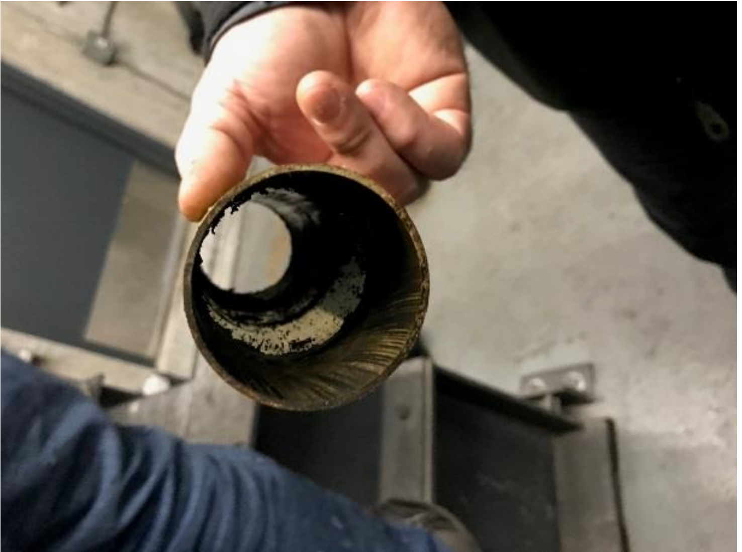
Photo 4 Brake brass sleeve with remnants of the rubber washer
