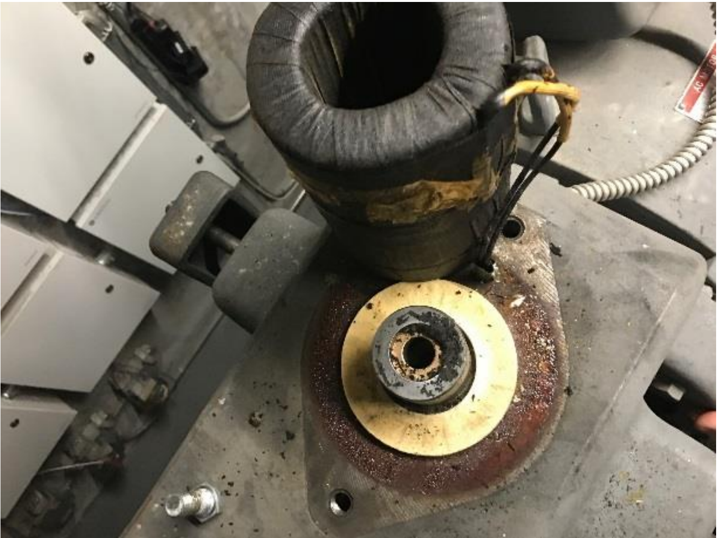
Photo 3 Machine brake assembly with rubber washer disintegrated to small pieces
