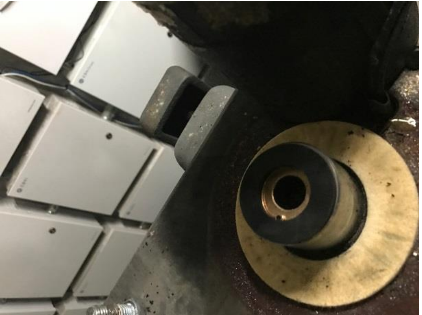
Photo 2 Machine brake assembly with a new rubber washer
