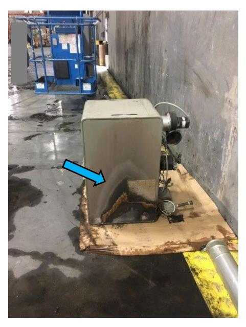
The flame pattern seen here suggest that a flame rollout occurred, causing the flames to lick the bottom and side of the heater.
