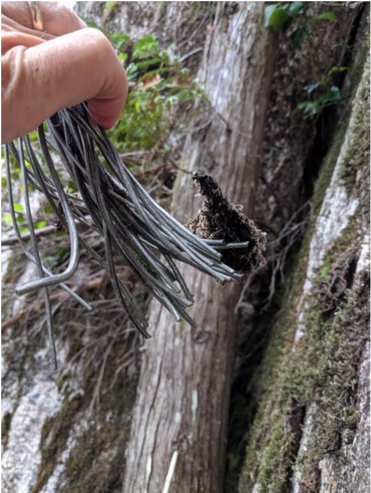
Image 4: Portion of separated haul rope end found downhill of tower ■.
