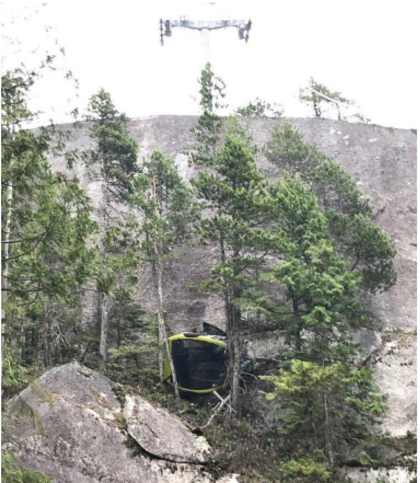
Image 5: View looking uphill at tower [REDACTED]. Damage and debris indicates gondola cabin likely struck tower/rock face after separation and haul rope was pulled out of cabin grip and past tower [REDACTED].
