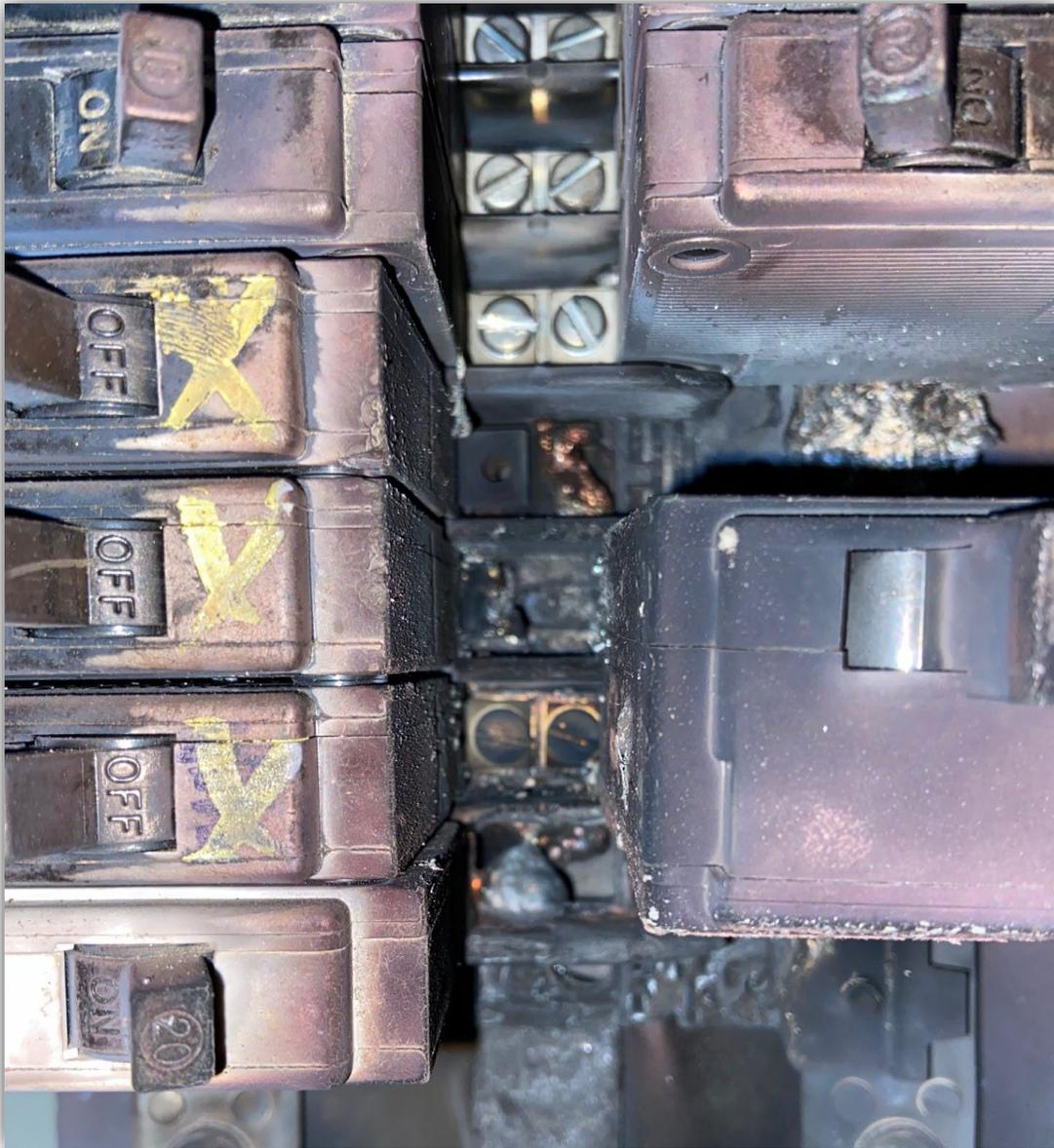
Image 2 – Closeup of the panel showing damage from the short circuit.
