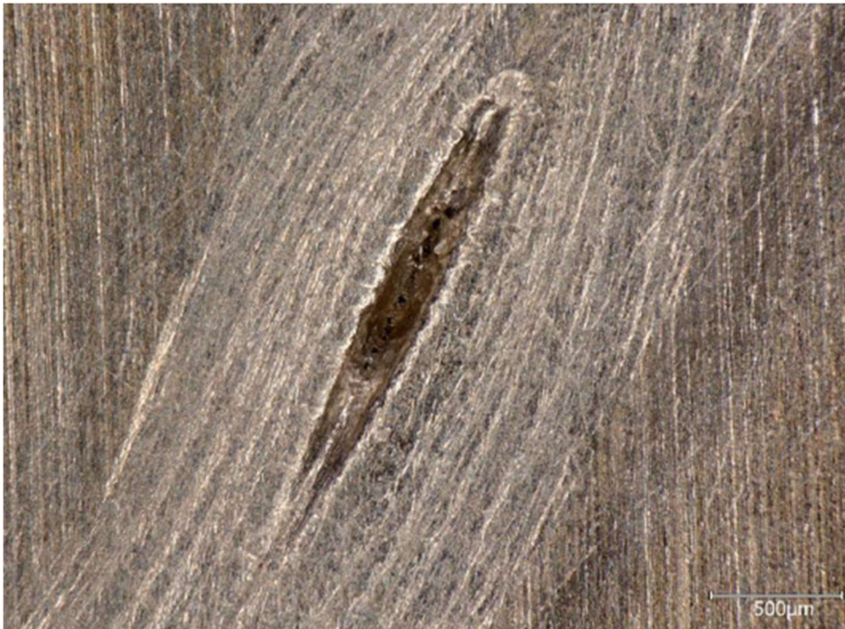
Figure 5: Electron microscope view of weld defect. Cassette 7B
