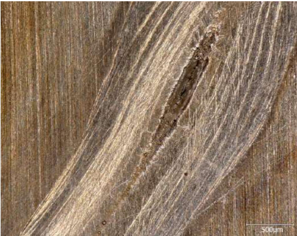
Figure 6: Electron microscope view of weld defect. Cassette 8B
