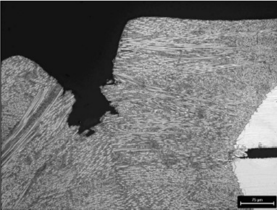
Figure 8: Defective weld after etching
