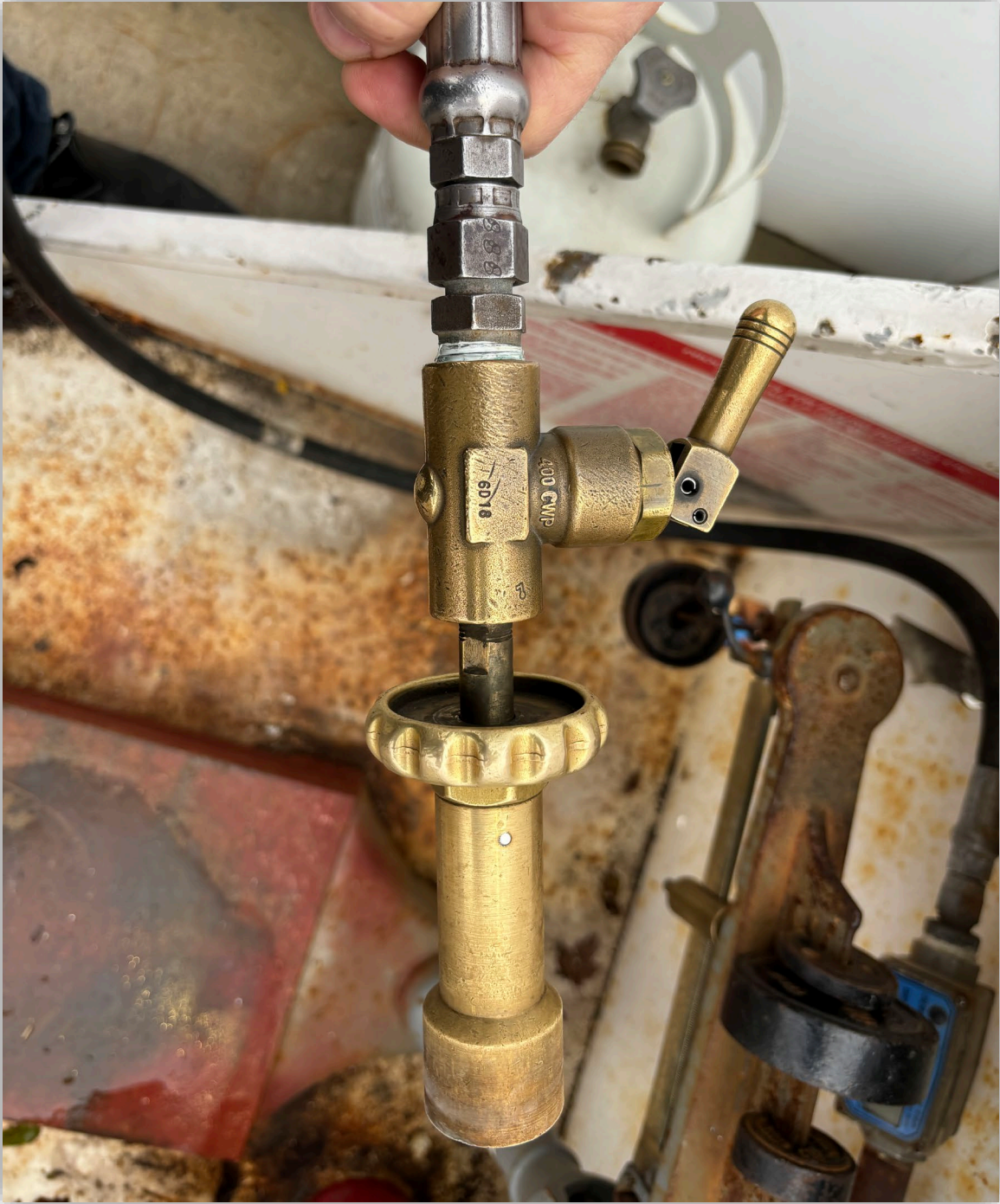
Image 7 - The propane filling nozzle, also without excess flow valve.
