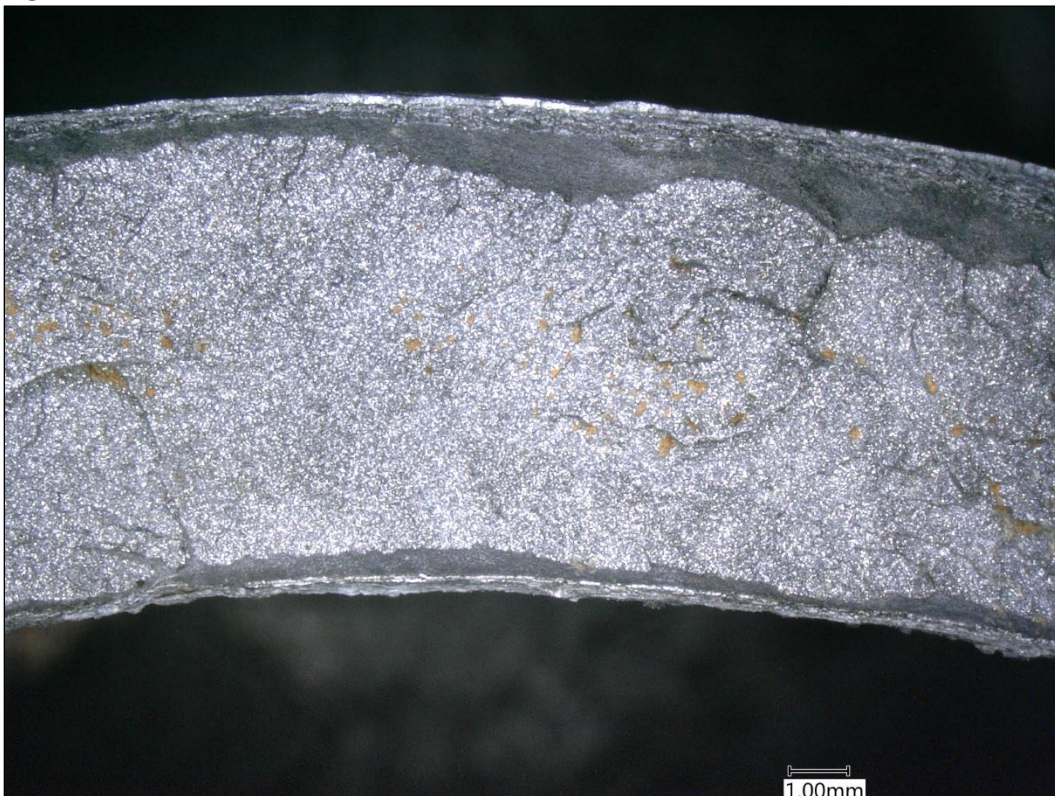
Figure 25 Reference 9 brittle fracture in overload zone
