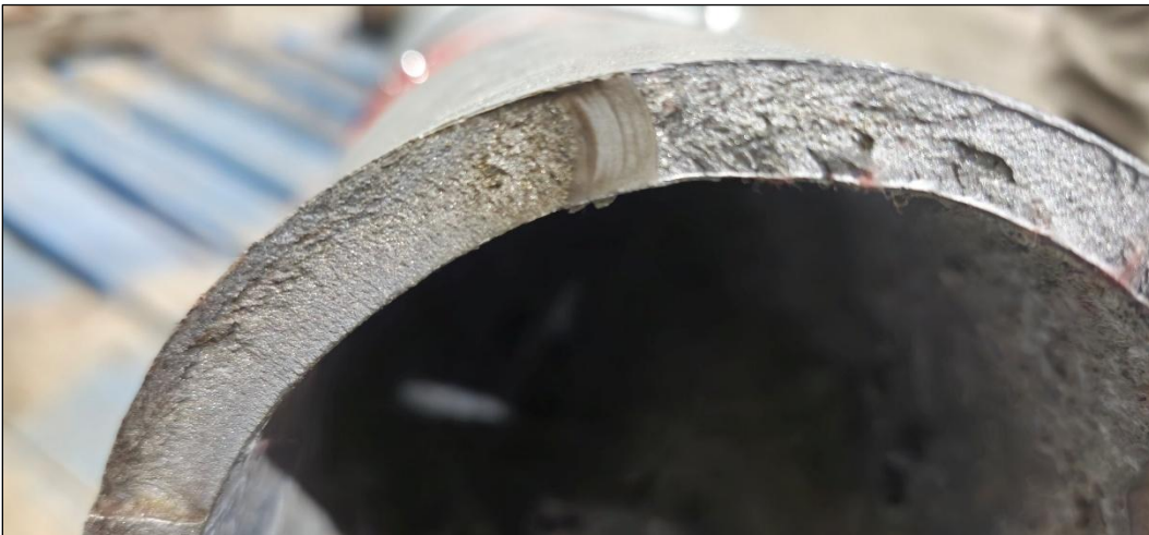
Figure 11 Fatigue crack initiation and growth on opposite side of thumbnail at the same relative location as the pipe weld fatigue crack. .
