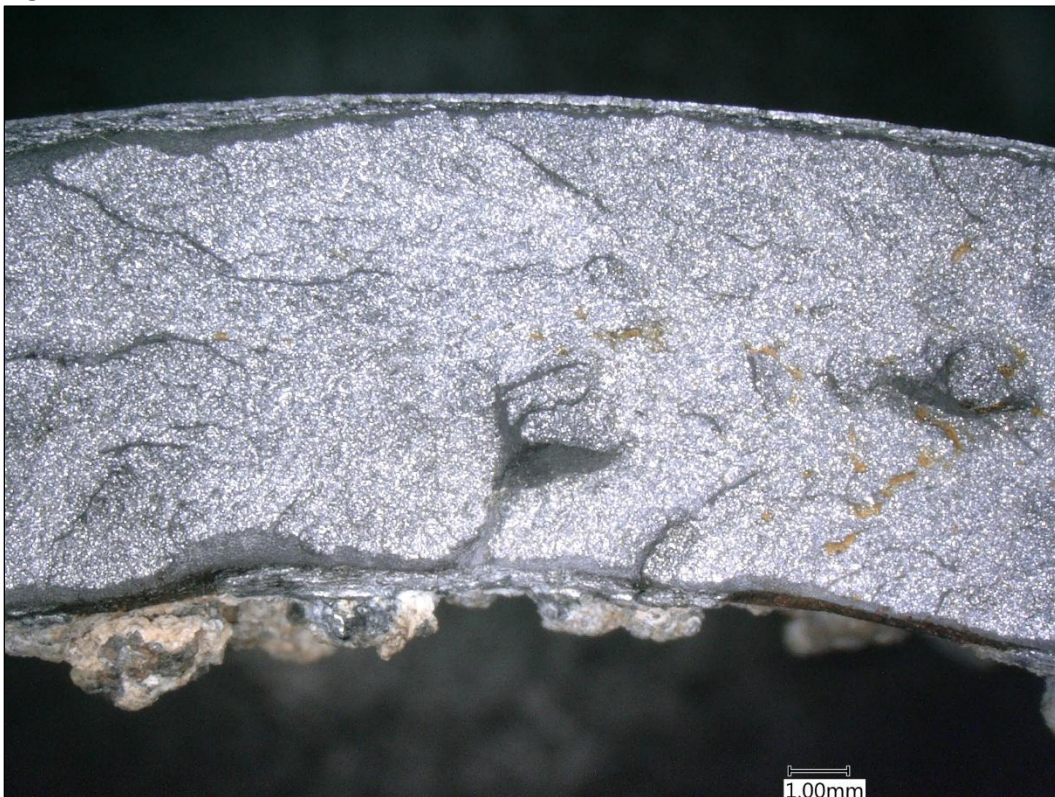
Figure 35 Reference 19 brittle fracture in overload zone.
