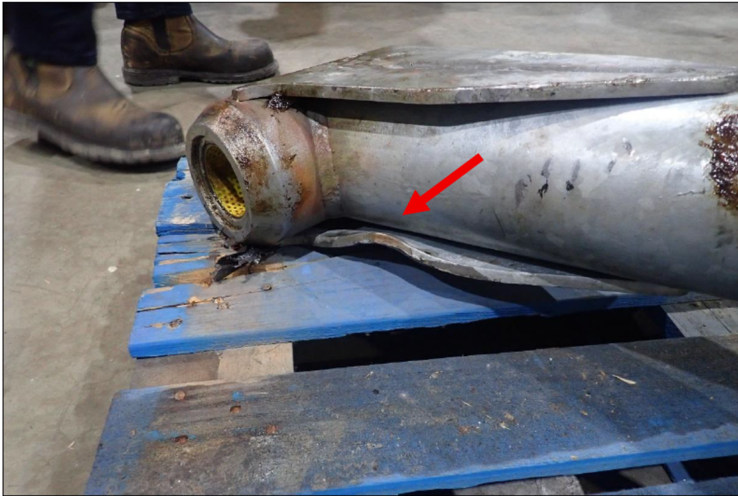
Figure 6 Deformation on upper reinforcing bracket cause by impact with lateral rail at drive station.
