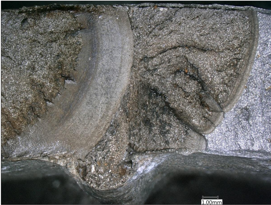
Figure 21 Reference 5 brittle fracture on either side of fatigue cracking through seam weld HAZ
