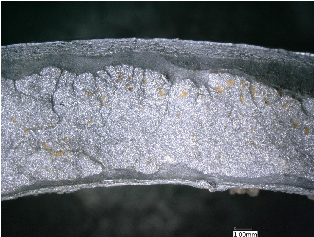
Figure 26 Reference 10 brittle fracture in overload zone
