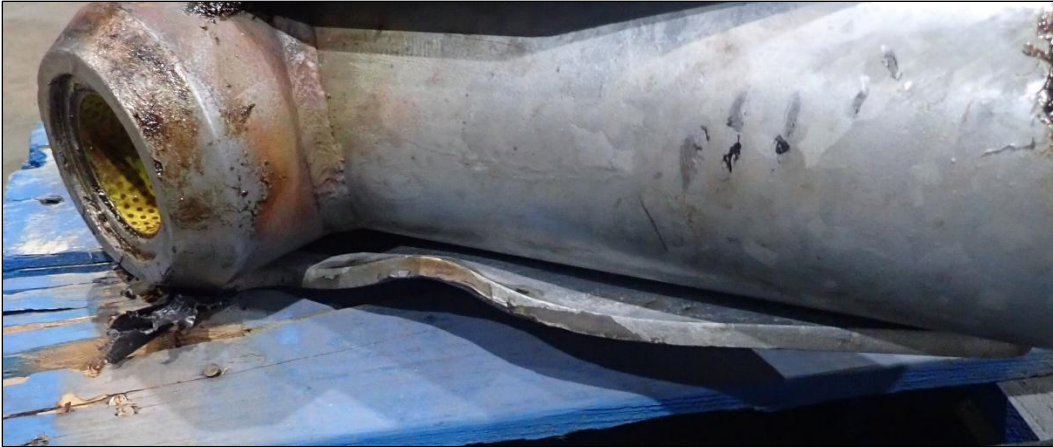
Figure 14 Close-up view of deformation in upper reinforcing bracket.
