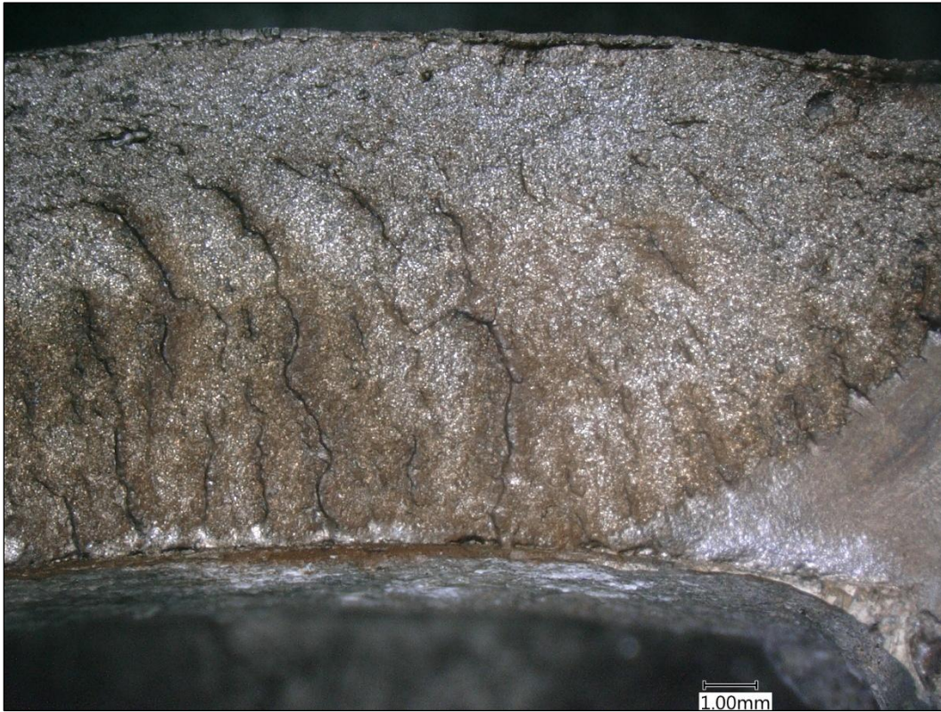
Figure 20 Reference 4 brittle fracture arrested at seam weld HAZ.
