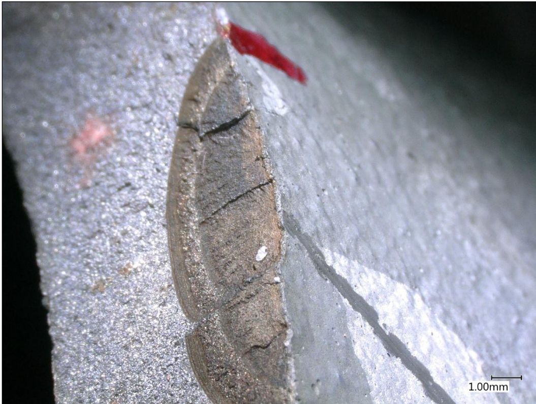
Figure 9 Close-up view of thumbnail area showing brittle fracture lines leading back to the thumbnail origin. The red mark is at the centerline of the intrados of the bend. The grey line is a scratch coming from the middle of the thumbnail (unknown origin).
