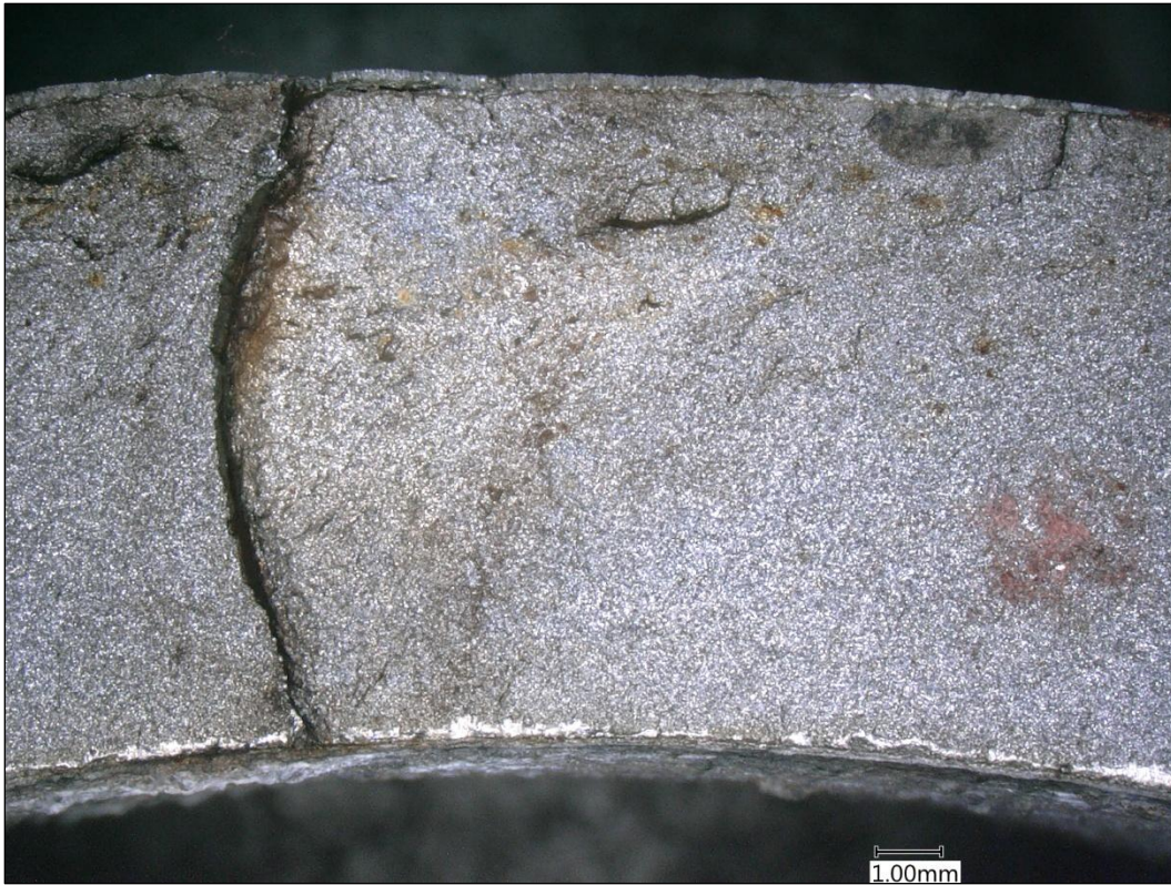
Figure 40 Brittle fracture near large thumbnail containing small thumbnail.
