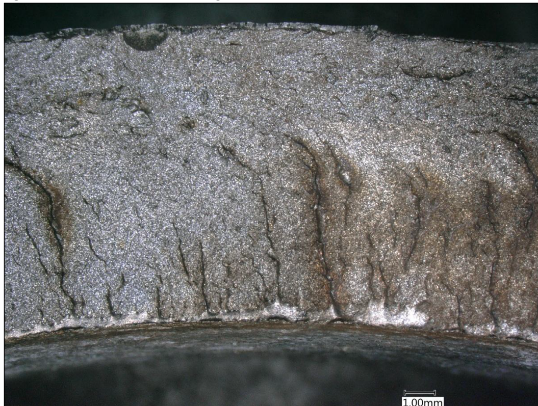
Figure 19 Reference 3 moving toward the seam weld (100% brittle)
