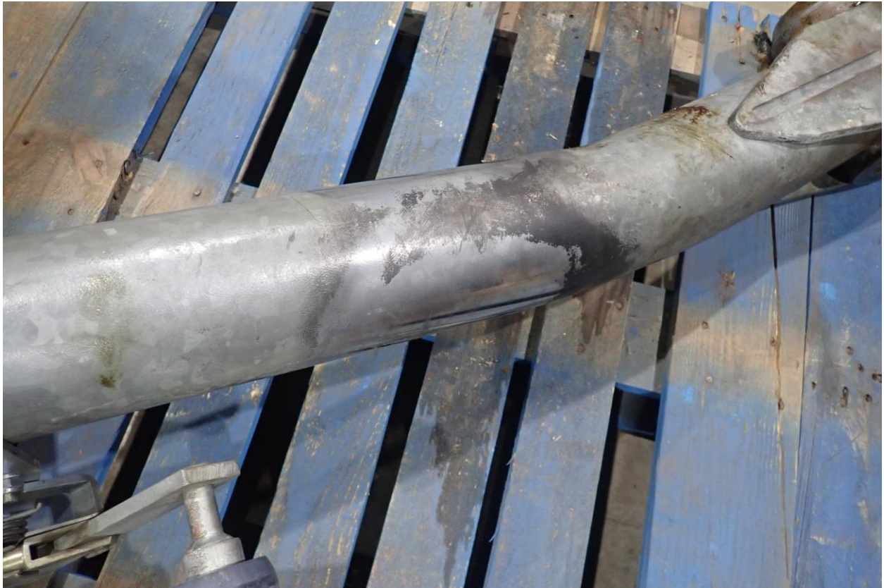
Figure 7 Shiny area on hanger arm galvanized surface indicating light contact during normal operation.
