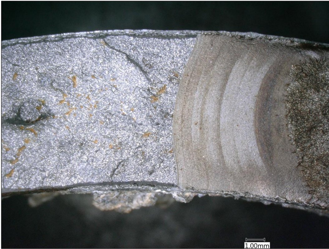
Figure 36 Reference 20 brittle fracture arrested . Beginning of fatigue crack at toe of brittle fracture zone. Position of fatigue zone roughly corresponds to position of HAZ fatigue zone on opposite side of thumbnail.
