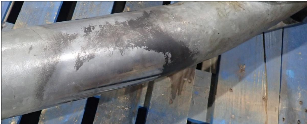
Figure 13 Shiny galvanizing from contact with unknown hardware during normal operations.
