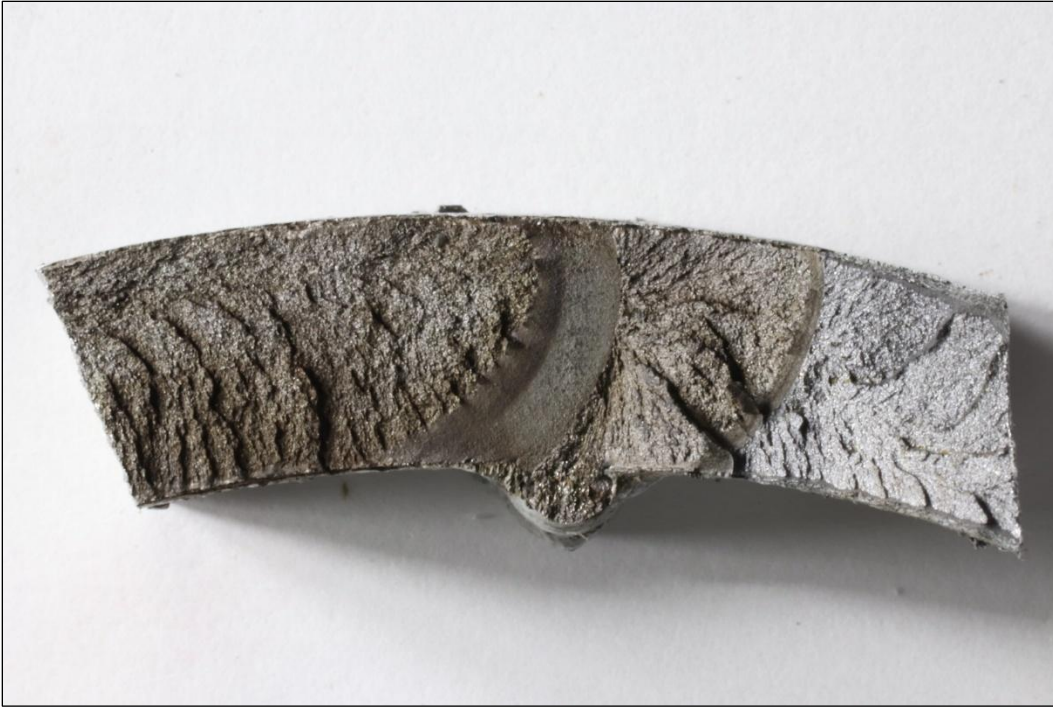
Figure 10 Crack arrest at the pipe seam weld. Fatigue crack grew until reaching a critical size and brittle cleavage proceeded. Microstructure change at weld arrested brittle fracture
