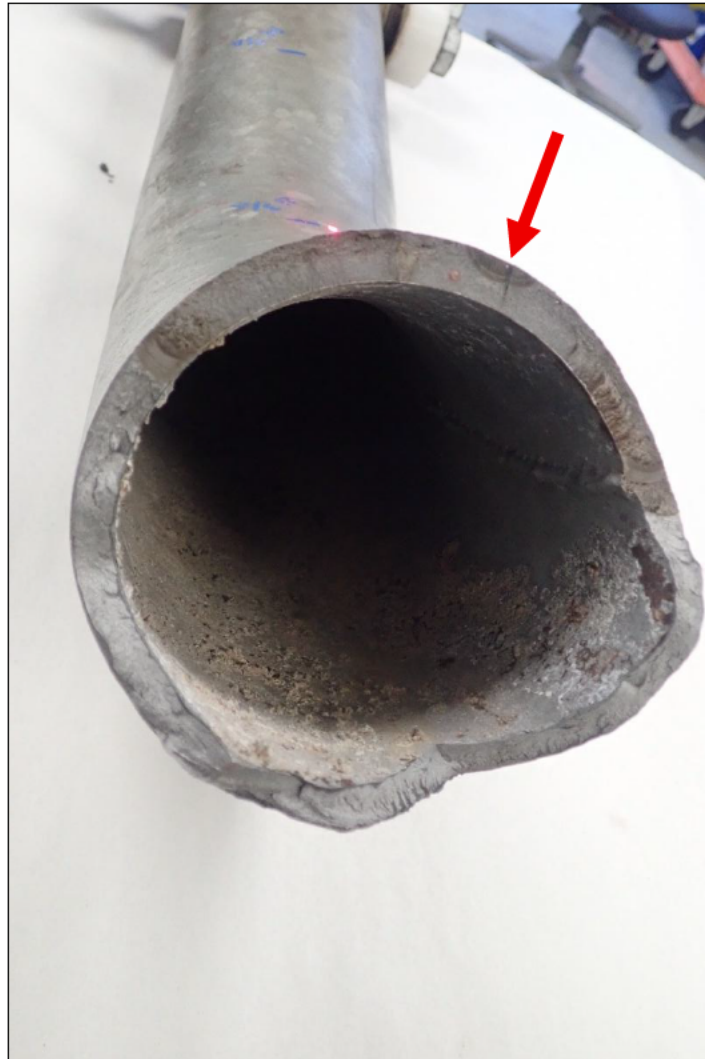
Figure 8 Thumbnail shaped fracture origin at roughly the 7 o'clock position from the intrados of the bend (intrados centerline at 6 O'clock position)
