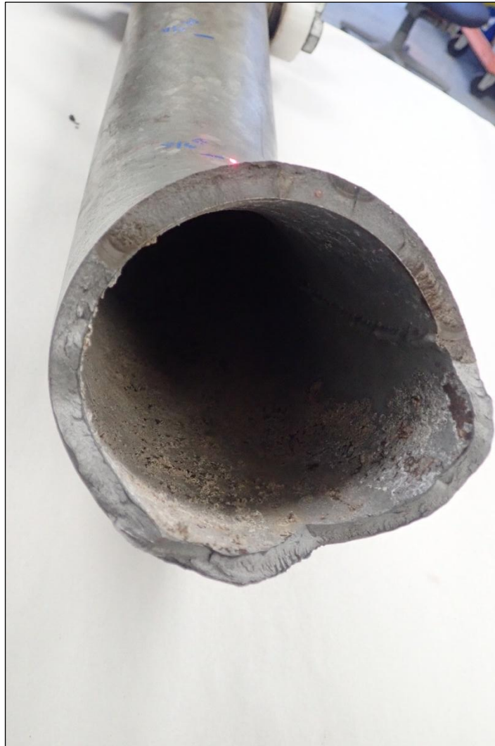
Figure 3 Overall view of the opposite side of the fracture (short 60° bend section) as it exists the gondola cover.
