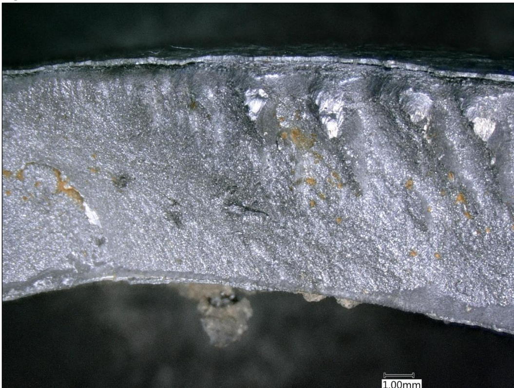
Figure 28 Reference 12 brittle fracture in overload zone.
