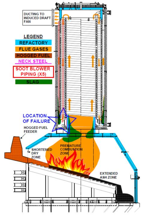
Premature combustion of hogged fuel, slag accumulations, and location of failure.
