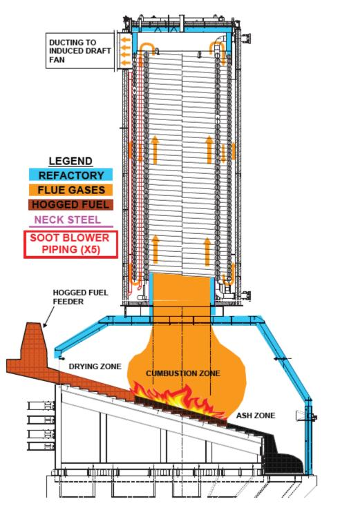
Normal combustion of hogged fuel reciprocating step-gate furnace and path of flue gases through helical coil heat exchanger.
