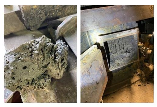
Slag (clinker) sample and deposit of slag on outer shell.
