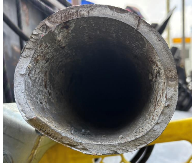
Figure 3 - Failure surface of the broken hanger, with fatigue markings visible at the '1 o'clock' position
