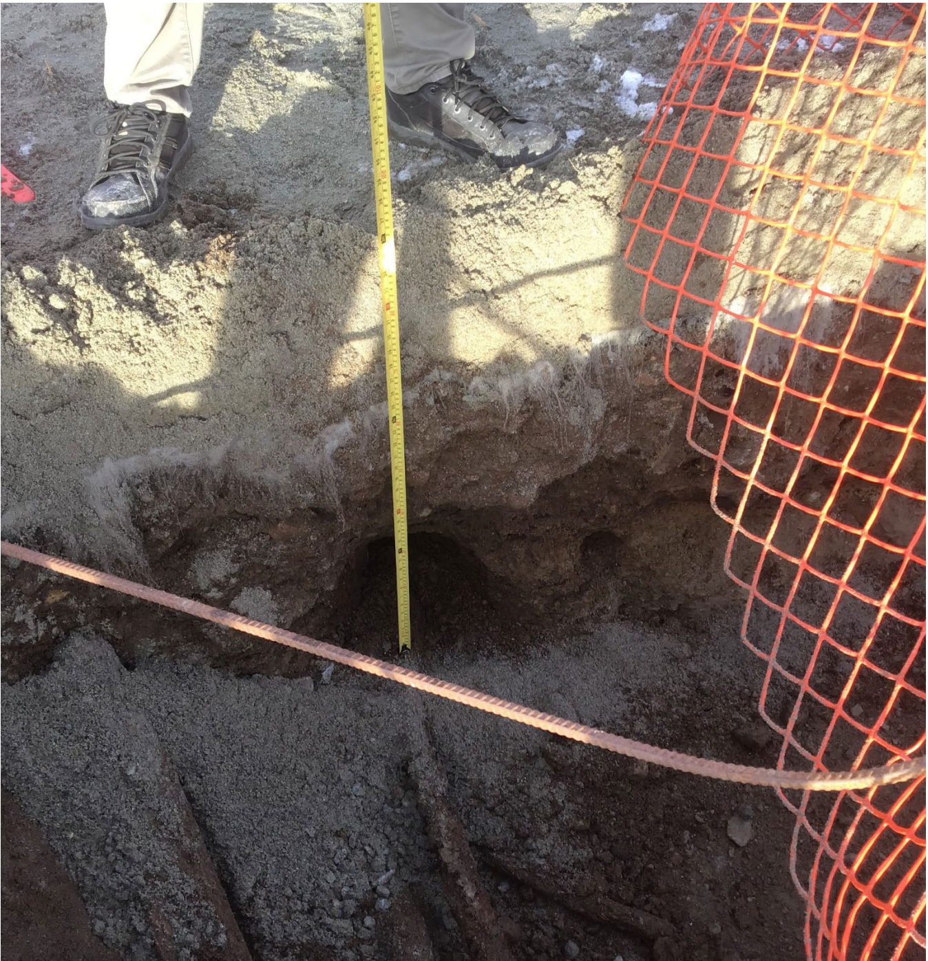
Image 4 - Test hole excavated away from roadway showing the cable was buried to proper 100cm depth but did not have any markings caution tape or mechanical protection.
