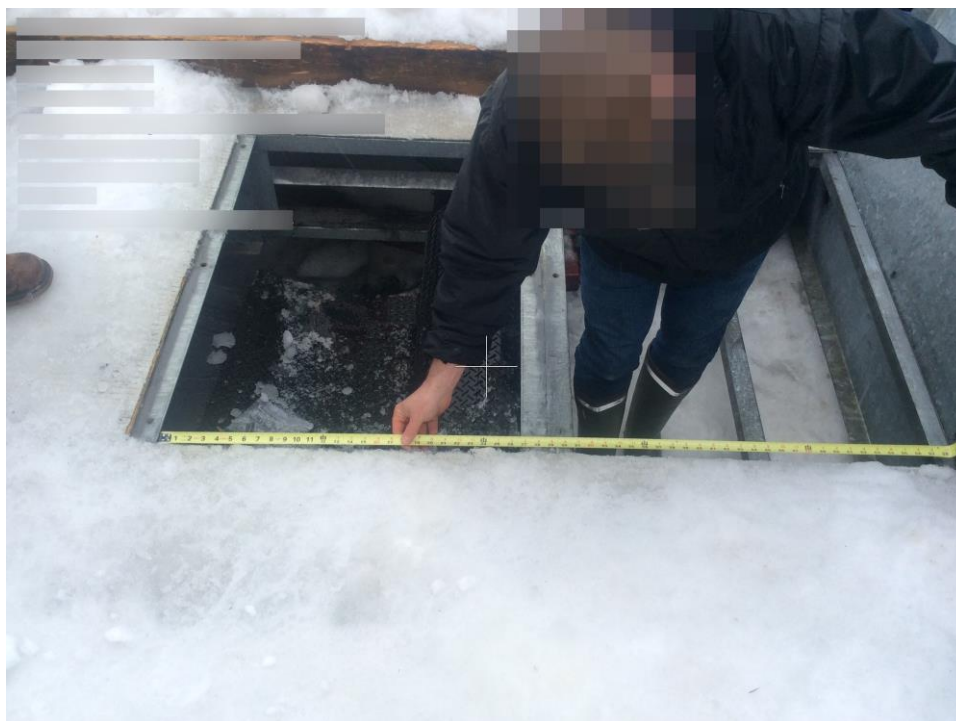
Figure 6: Tail unit, shows limited work space and tripping hazards when adjusting the belt.
