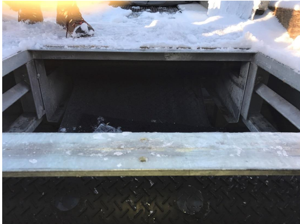
Figure 8: Belt entry where worker was found in equipment. Tripping hazard in foreground.
